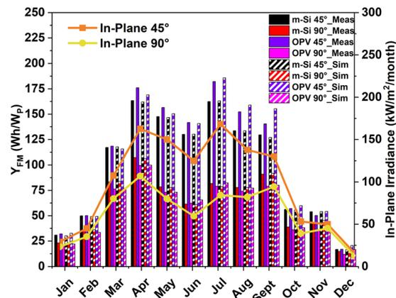
Fig. 4 Recorded monthly-specific-energy-yields ( $Y_{FM}$ ) of both OPV and m-Si modules over the year at 45° (m-Si #1 and OPV #1) and 90° (m-Si #2 and OPV #2) angles of inclination (solid columns). The respective simulated  $Y_{FM}$  of both module types at their respective outdoor inclinations over the year is represented by dashed columns of the same color. The recorded monthly in-plane irradiance over the year is represented by orange lines for 45° and yellow lines for 90°.
