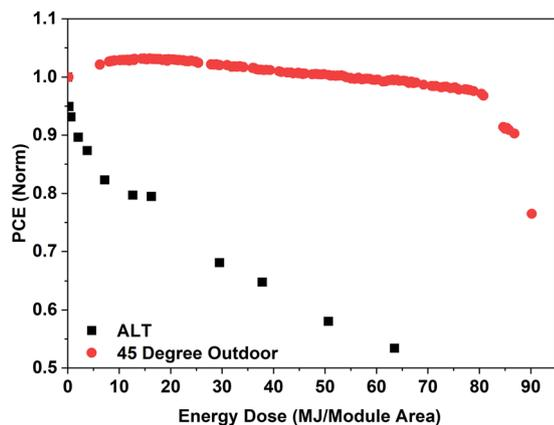
Fig. 5 PCE values, normalized to  $t_0$  performance, as a function of light energy dose incident onto the module surface in megajoules (MJ) during accelerated lifetime testing (black points) and during the one-year outdoor exposure at a  $45^\circ$  inclination angle (red points).
