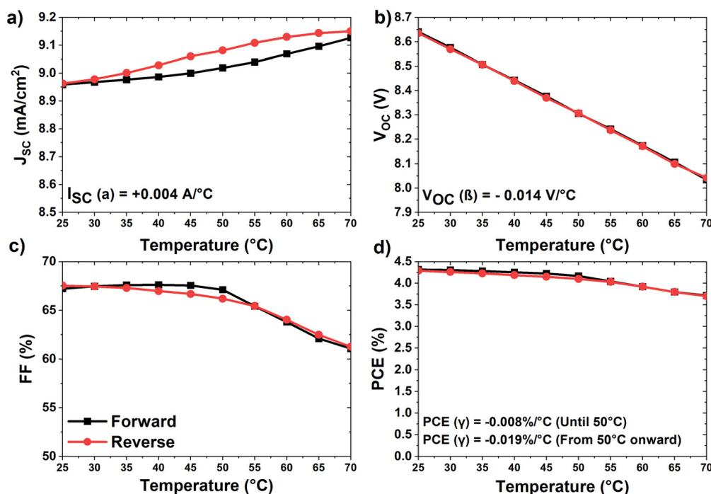
Fig. 2 Effect of temperature on the key photoelectrical parameters (a) temperature dependence of  $J_{SC}$ , (b) temperature dependence of  $V_{OC}$ , (c) temperature dependence of FF, and (d) temperature dependence of PCE) of the OPV module over a temperature range of 25–70 °C under AM1.5G conditions during upward (black) and downward (red) direction.
