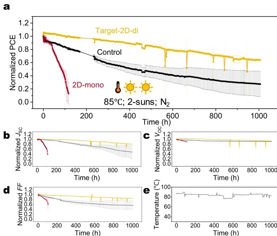
Fig. 6 Operational stability performance of control and target devices under 85 °C and 2-suns illumination: (a)–(d) normalized PCE,  $J_{sc}$ ,  $V_{oc}$ , and FF. Error bar represents the standard deviation of three individual devices. The data was normalized at 0.6 hour when the temperature increased to 85 °C. (e) The temperature profile during stability measurement.
