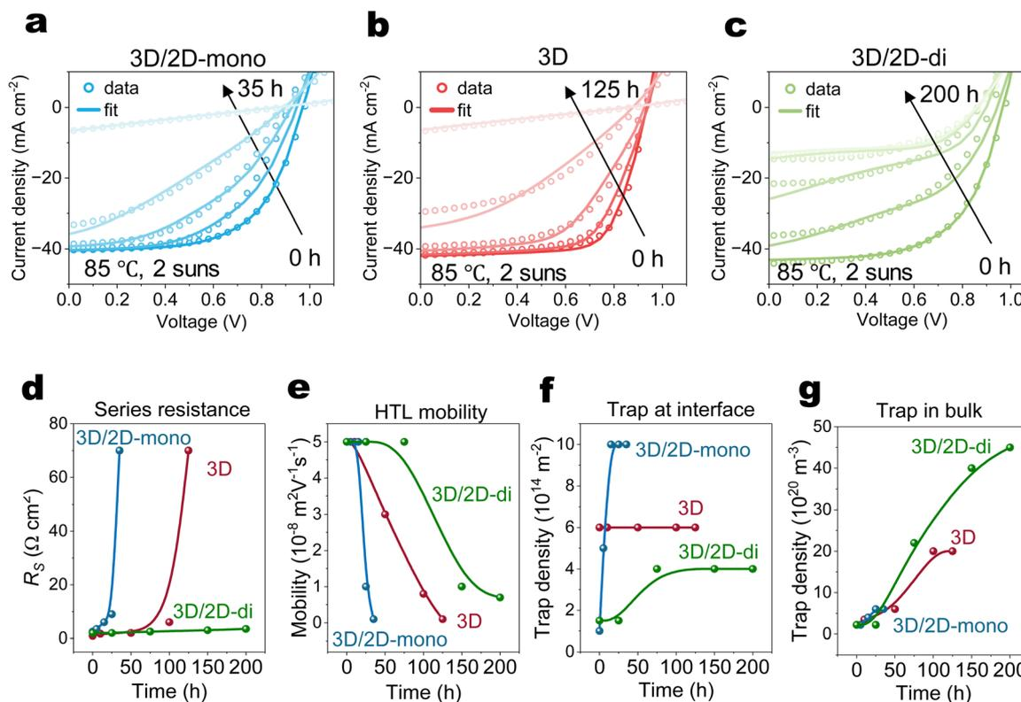
Fig. 4 Drift diffusion simulation results. (a)–(c) The experimental  $JV$  (open circles) and simulation fitting (solid line) of operational stability of 3D/2D-mono, 3D and 3D/2D-di devices under 85 °C and 2-sun illumination. (d)–(g) Corresponding simulation parameters obtained at various ageing time. The points in (d)–(g) are the values of the different parameters obtained by the simulation, while the connecting lines only show the trend and do not represent the simulated values.
