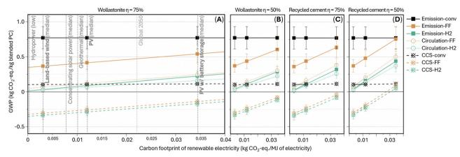
Fig. 7 Sensitivity analysis – influence of renewable electricity carbon footprint and electrolyzer energy efficiency on total GWP of conventional and electrochemical cement manufacturing schemes. The data point value is averaged GWP of the four blend designs, and the error bar shows the min-to-max range of the four values. 43,44
