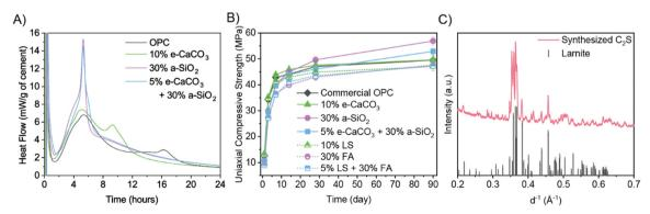
Fig. 4 (A) Calorimetry of 5 g of (blended) cement paste. (B) Compressive strength of (blended) cement paste using electrochemical products (e-CaCO<sub>3</sub> and a-SiO<sub>2</sub>) or conventional supplementary cementitious materials (limestone powder and fly ash) over 90 days. OPC = ordinary Portland cement; LS = limestone; FA = fly ash. (C) XRD of synthesized  $C_2S$  and reference.
