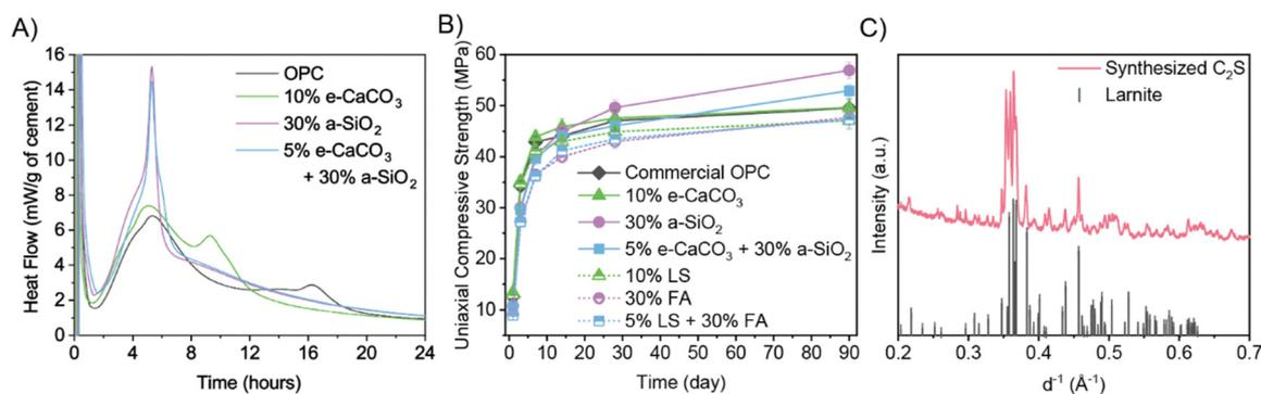
Fig. 4 (A) Calorimetry of 5 g of (blended) cement paste. (B) Compressive strength of (blended) cement paste using electrochemical products (e- $\text{CaCO}_3$  and a- $\text{SiO}_2$ ) or conventional supplementary cementitious materials (limestone powder and fly ash) over 90 days. OPC = ordinary Portland cement; LS = limestone; FA = fly ash. (C) XRD of synthesized  $\text{C}_2\text{S}$  and reference.
