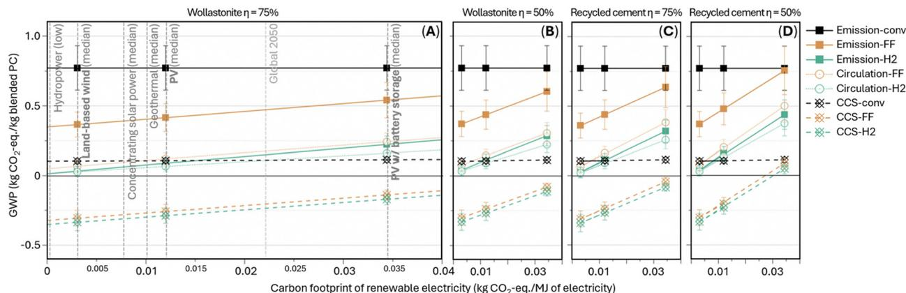
Fig. 7 Sensitivity analysis – influence of renewable electricity carbon footprint and electrolyzer energy efficiency on total GWP of conventional and electrochemical cement manufacturing schemes. The data point value is averaged GWP of the four blend designs, and the error bar shows the min-to-max range of the four values.<sup>43,44</sup>
