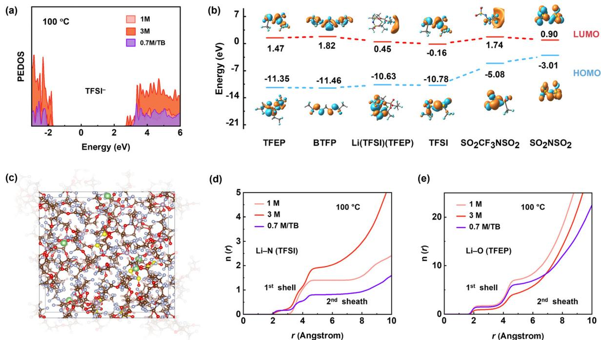
Fig. 5 AIMD simulations at 100 °C: the projected density of states (PDOS) of the TFSI<sup>-</sup> anion in different electrolytes. (b) LUMO and HOMO energies of the compositions and byproducts. (c) Snapshot of AIMD simulations of 0.7 M LiTFSI/TB. (d, f) The coordination number profiles of (e) Li-N<sub>TFSI</sub> and (f) Li-O<sub>TFEP</sub> for 1 M, 3 M LiTFSI/TFEP and 0.7 M LiTFSI/TB electrolytes.
