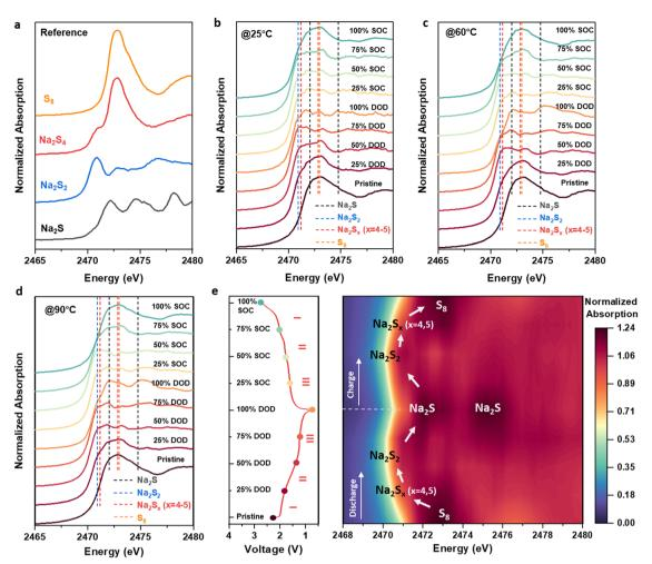
Fig. 4 Ex situ X-ray absorption spectroscopy (XAS) investigation of ASSSBs. (a) S K-edge XANES spectra of Na<sub>2</sub>S<sub>4</sub>, Na<sub>2</sub>S<sub>2</sub>, Na<sub>2</sub>S<sub>4</sub>, and S. Ex situ S K-edge XANES measurements for the ASSSBs operated at (b) 25 °C, (c) 60 °C, and (d) 90 °C. (e) The voltage profile and intensity mapping of the ex situ S K-edge XANES of the cell operated at 90 °C
