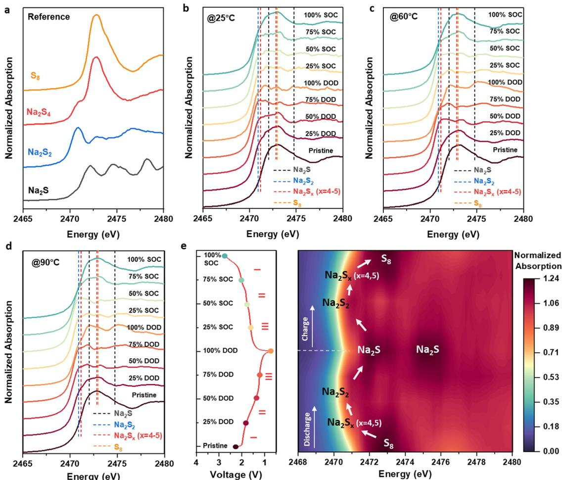
Fig. 4 *Ex situ* X-ray absorption spectroscopy (XAS) investigation of ASSSBs. (a) S K-edge XANES spectra of  $\text{Na}_2\text{S}$ ,  $\text{Na}_2\text{S}_2$ ,  $\text{Na}_2\text{S}_4$ , and  $\text{S}_8$ . *Ex situ* S K-edge XANES measurements for the ASSSBs operated at (b) 25 °C, (c) 60 °C, and (d) 90 °C. (e) The voltage profile and intensity mapping of the *ex situ* S K-edge XANES of the cell operated at 90 °C.
