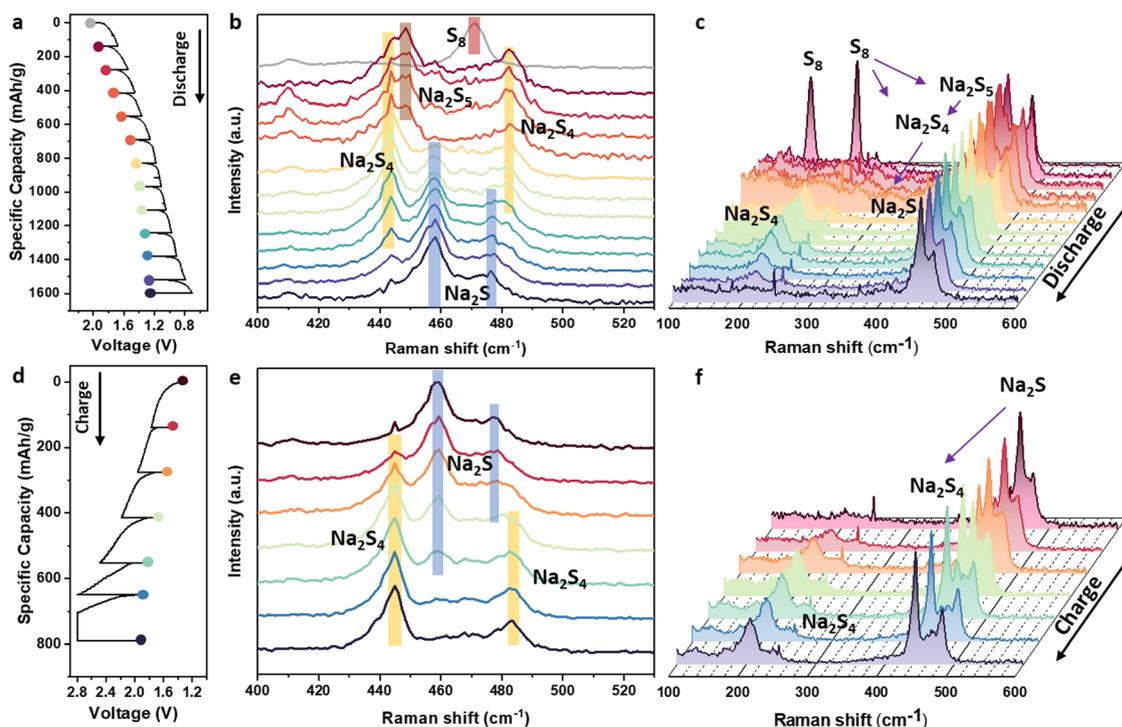
Fig. 5 *In situ* Raman investigation of the ASSSBs operated at room temperature. (a) Voltage profiles, (b) Raman spectra and (c) waterfall plot of the Raman spectra of the discharging process. (d) voltage profiles, (e) Raman spectra and (f) waterfall plot of the Raman spectra of the charging process.
