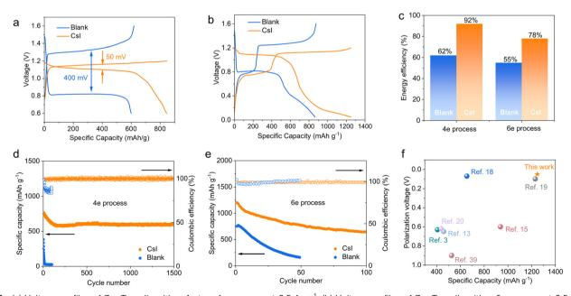
Fig. 5 (a) Voltage profiles of Zn-Te cells with a 4e transfer process at 0.5 A g<sup>-1</sup>. (b) Voltage profiles of Zn-Te cells with a 6e process at 0.5 A g<sup>-1</sup>. (c) Energy efficiencies of Zn-Te cells with different electrolytes. (d) and (e) Long-term cycling performance of Zn-Te cells. (f) The comparison of discharge capacity and polarization of various Zn-Te cells.
