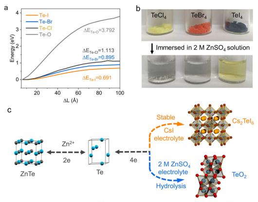
Fig. 1 (a) Dissociation energies for different bonding modes. (b) Visualization of the stability of TeX4 in blank electrolyte. (c) Schematic illustration of the conversion paths of Te electrode in different aqueous media.
