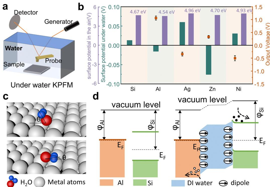
**Fig. 5** The influence of EDL on the work function of metals. (a) The diagram of the experimental setup of underwater KPFM. (b) The calculated surface potential under water, the surface potential of metal and Si in the air measured using KPFM, and the output voltage of the metal–Si wiping generator. (c) The principle of the surface potential of metals changes. (d) Band diagram of Schottky variations under water excitation.
