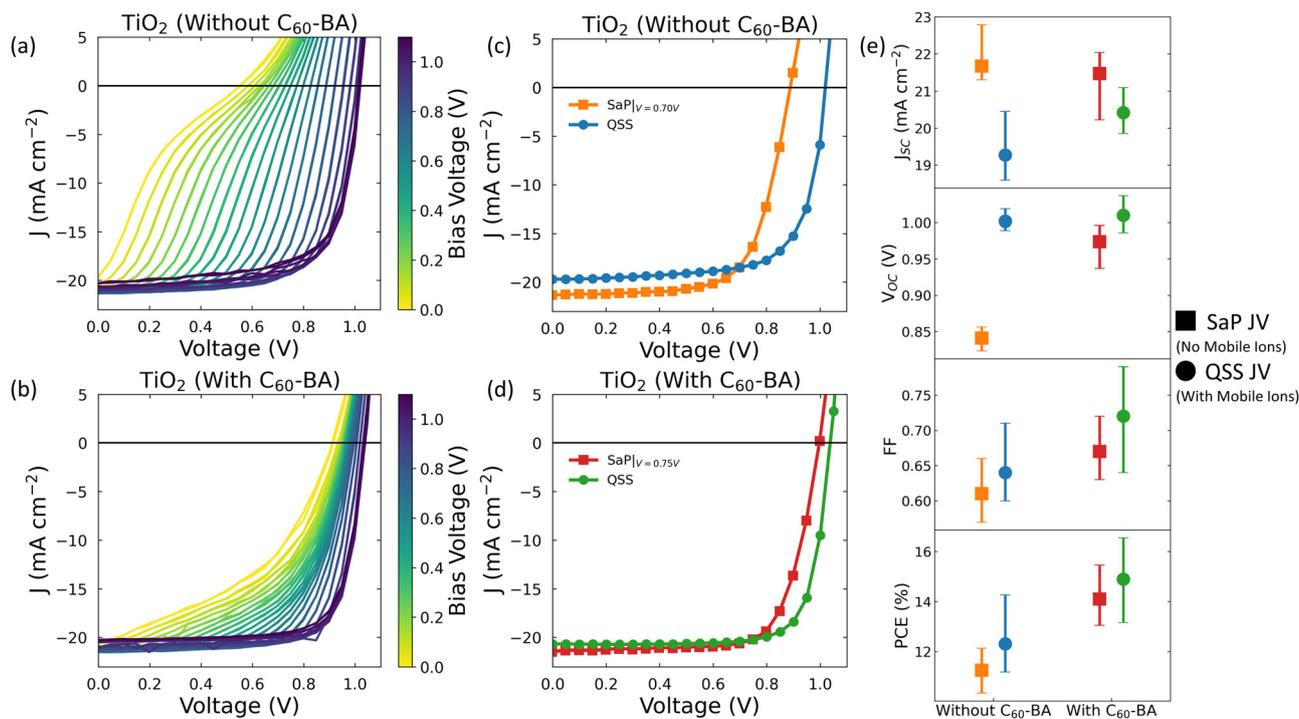
Fig. 2 Stabilise and Pulse measurement for the devices (a) without and (b) with C<sub>60</sub>-BA. The quasi-steady state (QSS)  $JVs$  and Stabilise and Pulse (SaP)  $JVs$  evaluated at  $V \approx V_{\text{flat}}$  for the TiO<sub>2</sub> devices (c) without and (d) with C<sub>60</sub>-BA. (e) Summary of the  $JV$  parameters extracted from the SaP  $JVs$  and QSS  $JVs$  for all measured devices. Error bars indicate the range of measured values.
