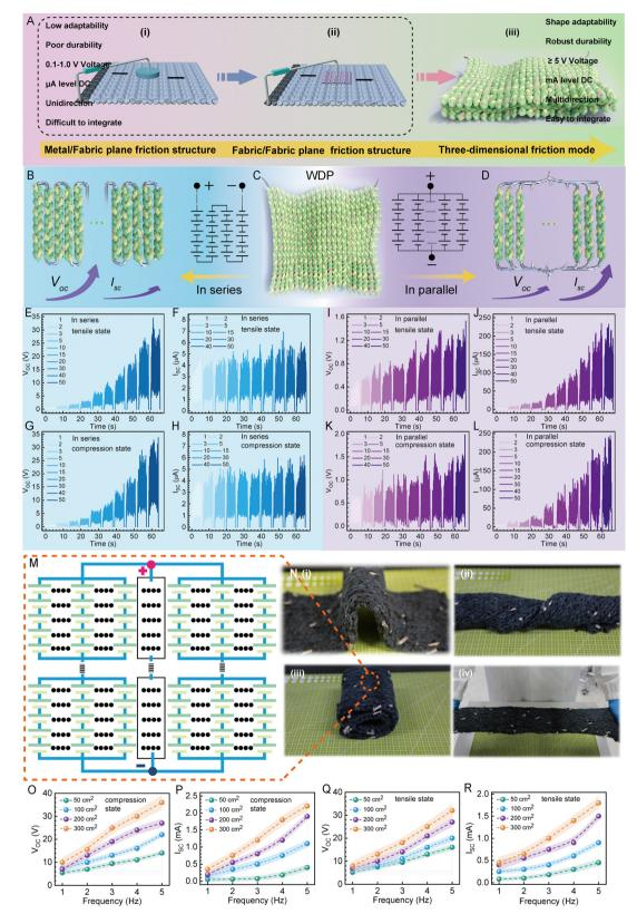
Fig. 2 Series/parallel characteristics and weaving design. (A) Advantages of the 3D friction model compared with the plane friction model. (B)-(D) Schematic diagram of SFs series and parallel connections. (E)–(H) Electrical properties of SFs in series. (I)–(L) Electrical properties of SFs in parallel. (M) and (N) Design structure and optical photos of WDPs. (O)–(R)  $V_{oc}$  and  $I_{sc}$  of SFs under different areas and frequencies.
