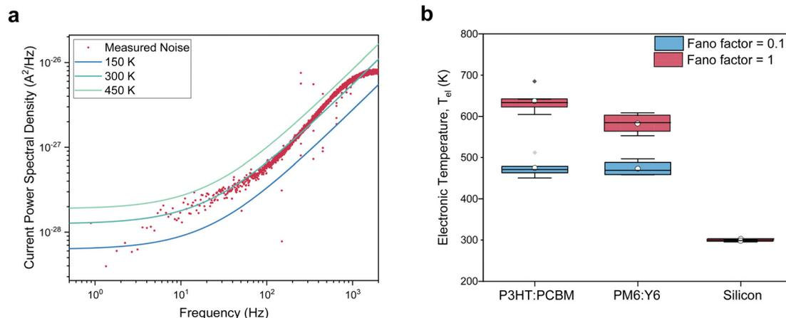
**Fig. 3** Electronic temperature in the dark and under illumination. (a) Noise spectra of a PM6:Y6 solar cell in the dark at room temperature and  $V = 0$ . The colored lines are the predicted thermal noise with different electronic temperatures. A temperature of  $\sim 300$  K best fits the noise spectra. (b) Extracted electronic temperatures under open-circuit conditions for different solar cells under sub-1 Sun illumination intensity at room temperature.
