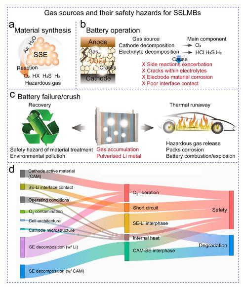
Fig. 4 (a)-(c) Gas sources and corresponding safety hazards for SSLMBs. (d) Safety landscape for SSLMBs. Reproduced with permission from ref. 52.
