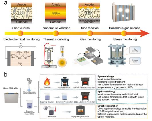
Fig. 9 (a) Potential safety hazards and corresponding monitoring means for SSLMBs. Reproduced with permission from ref. 136 and 141-143. (b) Overview of feasibility and challenges of different recycling technologies for SSLMBs. Reproduced with permission from ref. 144.
