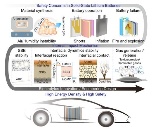
Fig. 1 Schematic representation of challenges for SSLMBs
