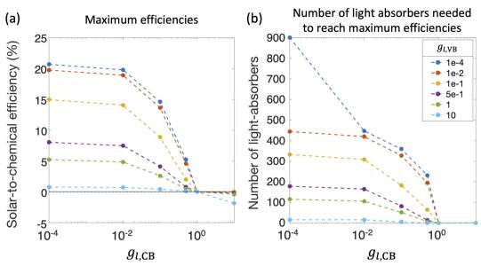
Fig. 8 (a) Maximum solar-to-chemical (STC) efficiencies and (b) corresponding number of light absorbers as a function of asymmetry factors in limiting current density for redox shuttle reduction,  $g_{l,CB}$  and  $H_2$  oxidation,  $g_{l,VB}$ . For all plots,  $j_{l,RS,a}/j_{sc,N=1}=1\times10^{-2}$ ,  $j_{0,RS}=10$  A m<sup>-2</sup>,  $\alpha_{a,RS}=0.5$ ,  $j_{0,H2}=10$  A m<sup>-2</sup> and  $\alpha_{a,H2}=1$ .
