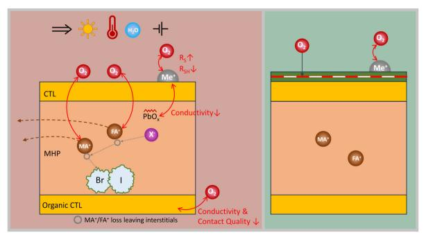
Fig. 8 Organic components can be removed from MHP due to oxidation of MA<sup>+</sup> or FA<sup>+</sup>. The resulting interstitials enhance halide segregation. Additionally, oxygen can react with Pb, with the metal electrodes or CTLs negatively impacting conductivity, stability and/or contact quality
