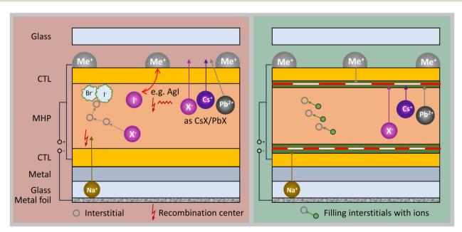
Fig. 12 PID leads to ion movement, especially of Na<sup>+</sup>, causing instabilities in the PSC. This can be mitigated by introducing ion blocking layers or by reducing ion migration due to filling of interstitials.
