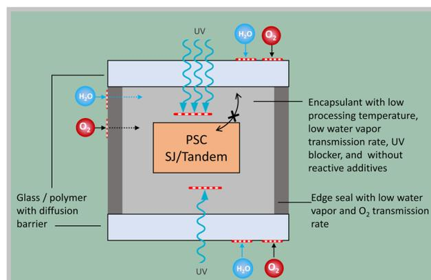
Fig. 11 Module packaging with glass–glass or backsheets with diffusion barriers protect SJ PSCs or MHP/Si tandem solar cells from water vapor and oxygen. An edge sealing and encapsulation material with low WVTR and low oxygen transmission rates prevent water and oxygen ingress from the side. The encapsulation material needs to be unreactive with MHPs and be processable at low temperatures.
