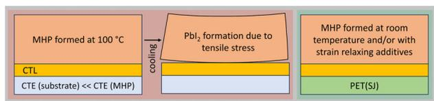
**Fig. 6** MHP formation at elevated temperatures on substrates with significantly lower CTE than MHP (like Si and glass) results in tensile stress within the MHP layer that leads to PbI<sub>2</sub> formation over time. Furthermore, stress can be decreased by MHP formation at room temperature and for SJ PSCs on PET substrates.
