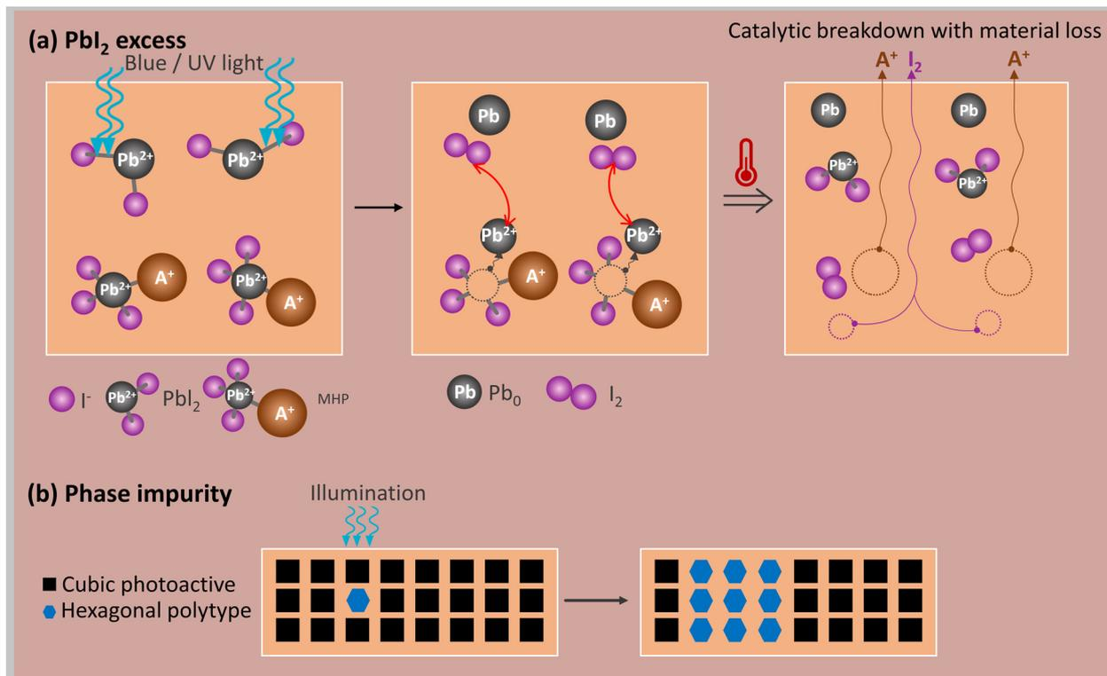
Fig. 2 (a)  $\text{PbI}_2$  residues absorbing blue/UV light can initiate a catalytic breakdown reaction with material loss in the form of  $\text{A}^+$  and  $\text{I}_2$ . (b) Nanoscale hexagonal polytypes acting as nucleation sites for further degradation of cubic photoactive to hexagonal not photoactive phase.
