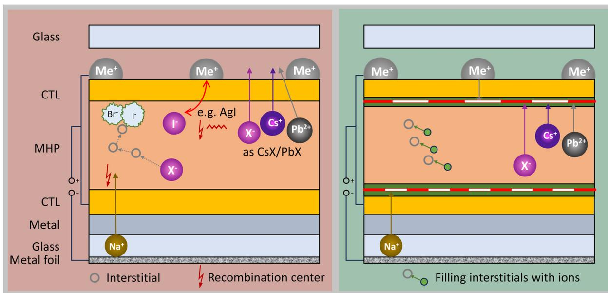
Fig. 12 PID leads to ion movement, especially of Na<sup>+</sup>, causing instabilities in the PSC. This can be mitigated by introducing ion blocking layers or by reducing ion migration due to filling of interstitials.
