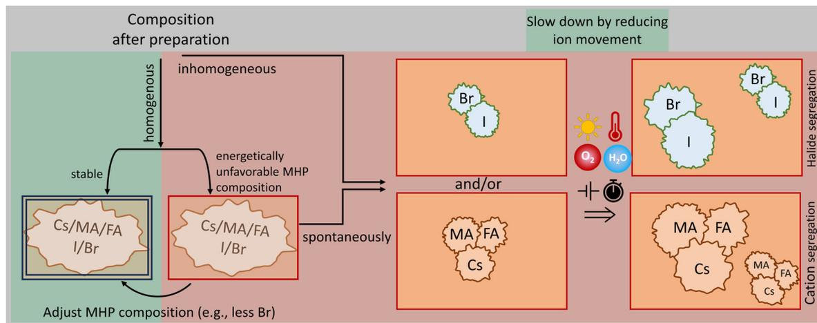
Fig. 3 Phase segregation in mixed cation and/or halide MHP films can either occur directly at MHP formation due to inhomogeneous mixing during preparation or spontaneously if the composition is energetically unfavourable (at certain temperatures). In both cases, phase segregation will proceed with time and be accelerated by external influences whereas (halide) segregation can be slowed down by reducing ion movement.
