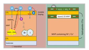
Fig. 7 Water vapor can react with the MHP resulting in decomposition in, among others, PbX<sub>2</sub> visible by a yellow colour. Decomposition products are highly reactive with metal electrodes. Furthermore, water vapor can induce instabilities in (doped) CTLs and moisture induced defects enhance ion movement resulting in halide segregation. Mitigation strategies are barrier layers, hydrophobic CTLs, (quasi) 2D MHP on top of 3D MHP and avoiding of MA+ or encapsulation (see Fig. 11).
