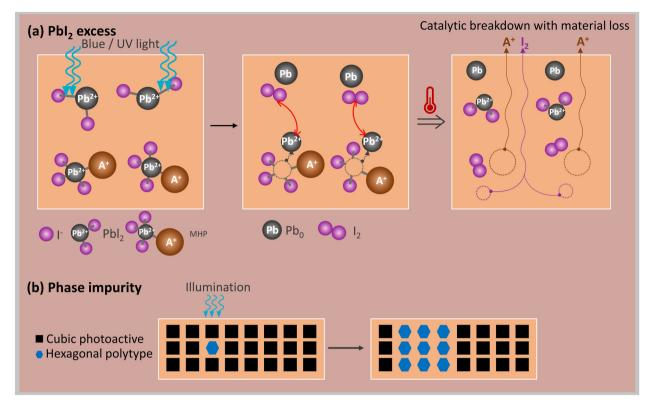
Fig. 2 (a) PbI<sub>2</sub> residues absorbing blue/UV light can initiate a catalytic breakdown reaction with material loss in the form of A<sup>+</sup> and I<sub>2</sub>. (b) Nanoscale hexagonal polytypes acting as nucleation sites for further degradation of cubic photoactive to hexagonal not photoactive phase
