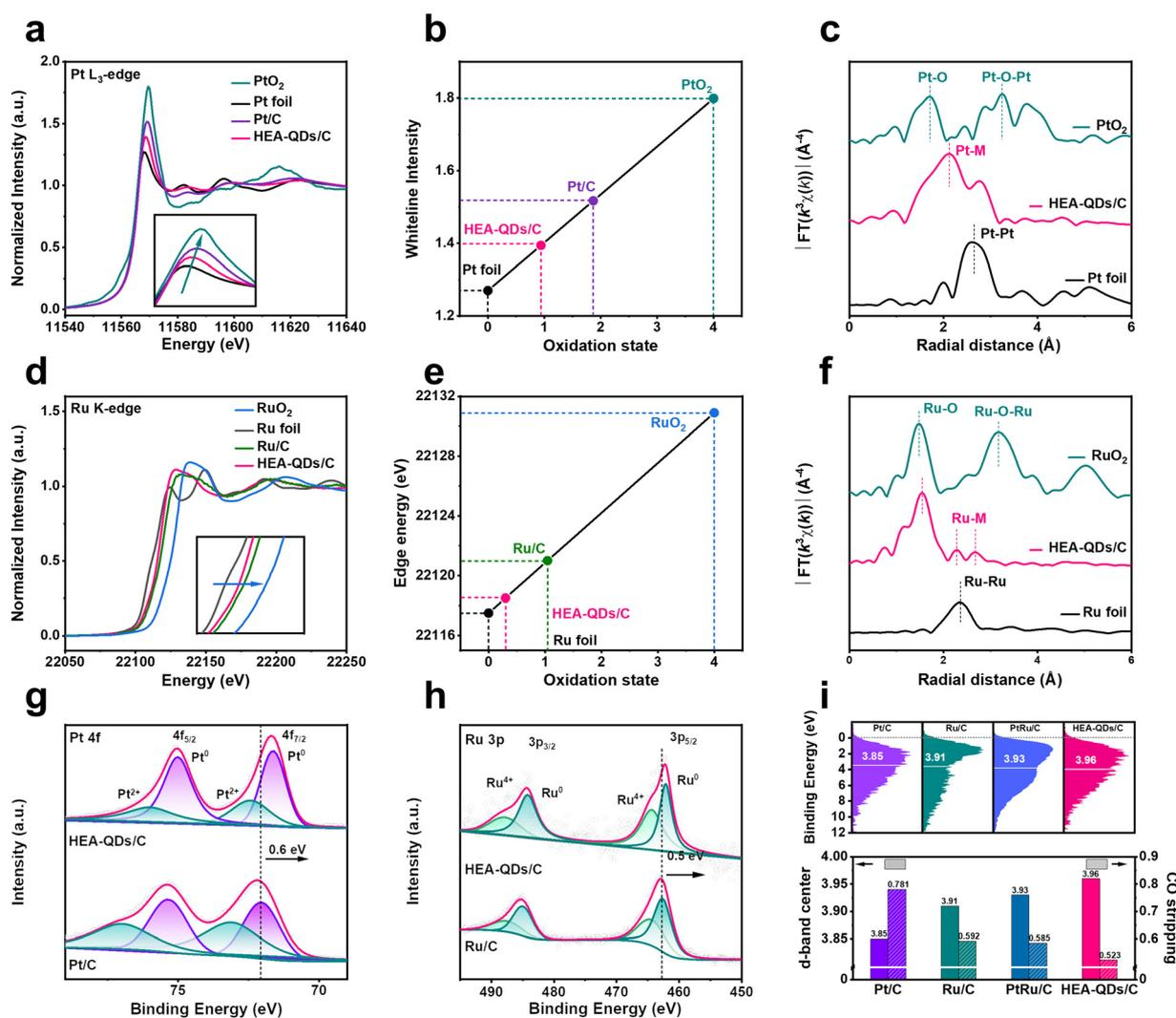
Fig. 2 Electronic and geometry structures analysis of HEA-QDs. (a) The XANES spectra of the Pt  $L_3$ -edge, (b) linear component fitting analysis and (c) FT-EXAFS spectra of Pt. (d) The XANES spectra of the Ru K-edge, (e) linear component fitting analysis and (f) FT-EXAFS spectra of Ru. (g) XPS spectra of Pt and (h) Ru. (i) VBS spectra (top) and CO oxidation peak potentials (down) of different catalysts.
