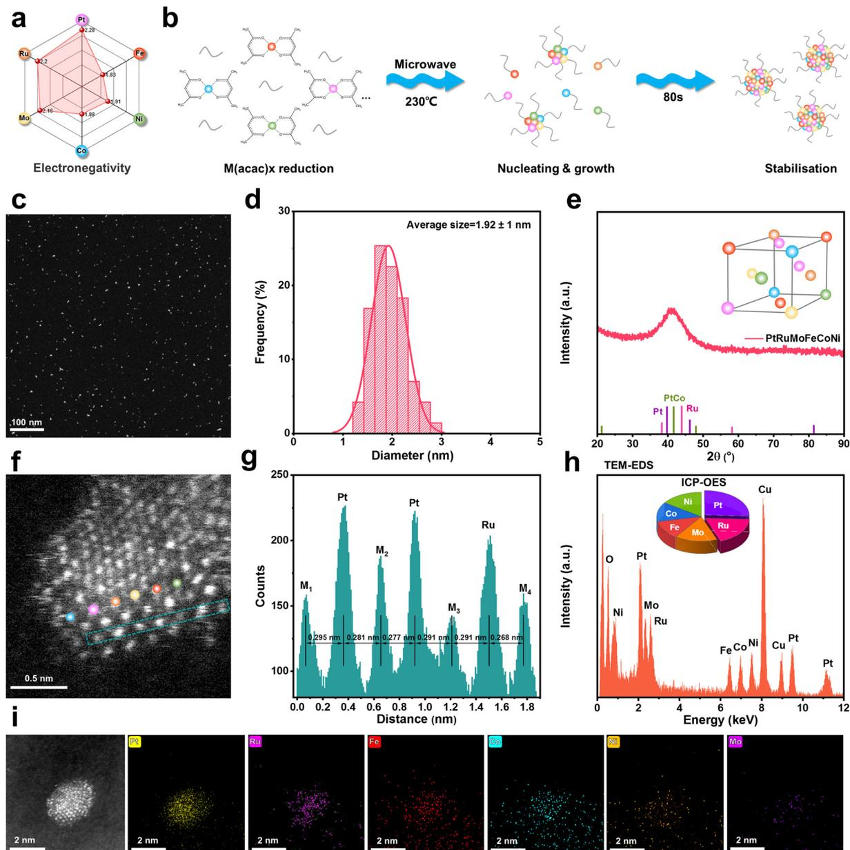
**Fig. 1** Morphology structure and composition characterization of HEA-QDs. (a) and (b) Preparation procedure. (c) HAADF-STEM image and corresponding (d) size distribution histogram. (e) XRD pattern. (f) AC-STEM image and (g) line profile along the dashed line in (f). (h) TEM-EDS and atomic ratio of different elements from the result of ICP-OES. (i) AC-STEM and corresponding STEM-EDS mapping images.
