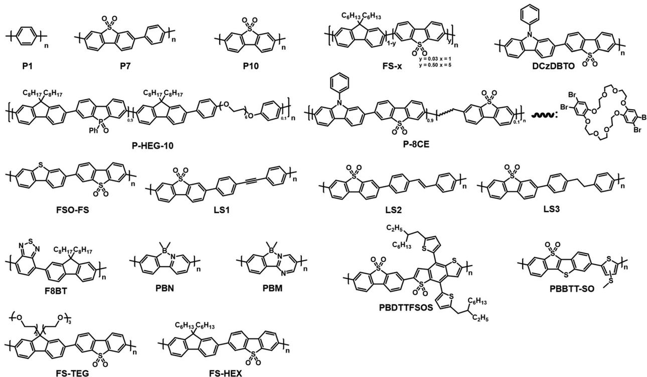
Scheme 1 Molecular structures of linear polymeric photocatalysts.
