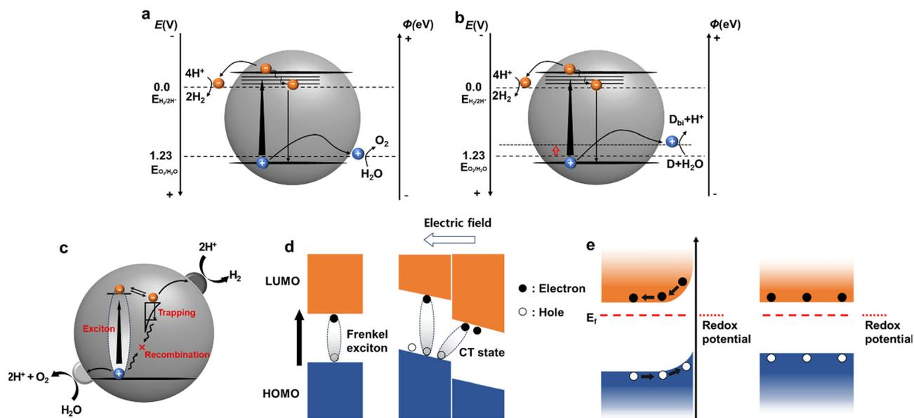
Fig. 2 Energy and potential diagrams of (a) photocatalytic overall water splitting and (b) half hydrogen reduction with a sacrificial donor (denoted as D). ( $\Phi = -eE$  (vs. NHE)  $-4.44$  eV,  $e$  is an elementary charge).  $D_{bi}$  means the biproduct in oxidation reaction of compound D. (c) Schematic of the photocatalytic redox reaction processes. (d) Exciton photogeneration at a single domain and heterojunction. (e) Band structures at different interface conditions.
