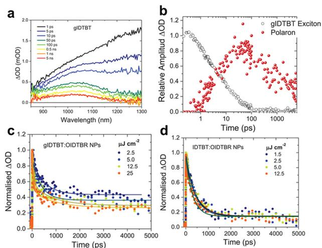
**Fig. 7** (a) TA spectra of the gIDTBT dispersion. (b) Deconvoluted transient absorption kinetics probed at 750 nm. Transient absorption kinetics at different fluences of (c) gIDTBT:ODTBR and (d) IDTBT:ODTBR. All transient absorption data were measured under 650 nm excitation using a 5  $\mu\text{J cm}^{-2}$  fluence. Reproduced with permission.<sup>92</sup> Copyright 2021, Wiley-VCH publication.
