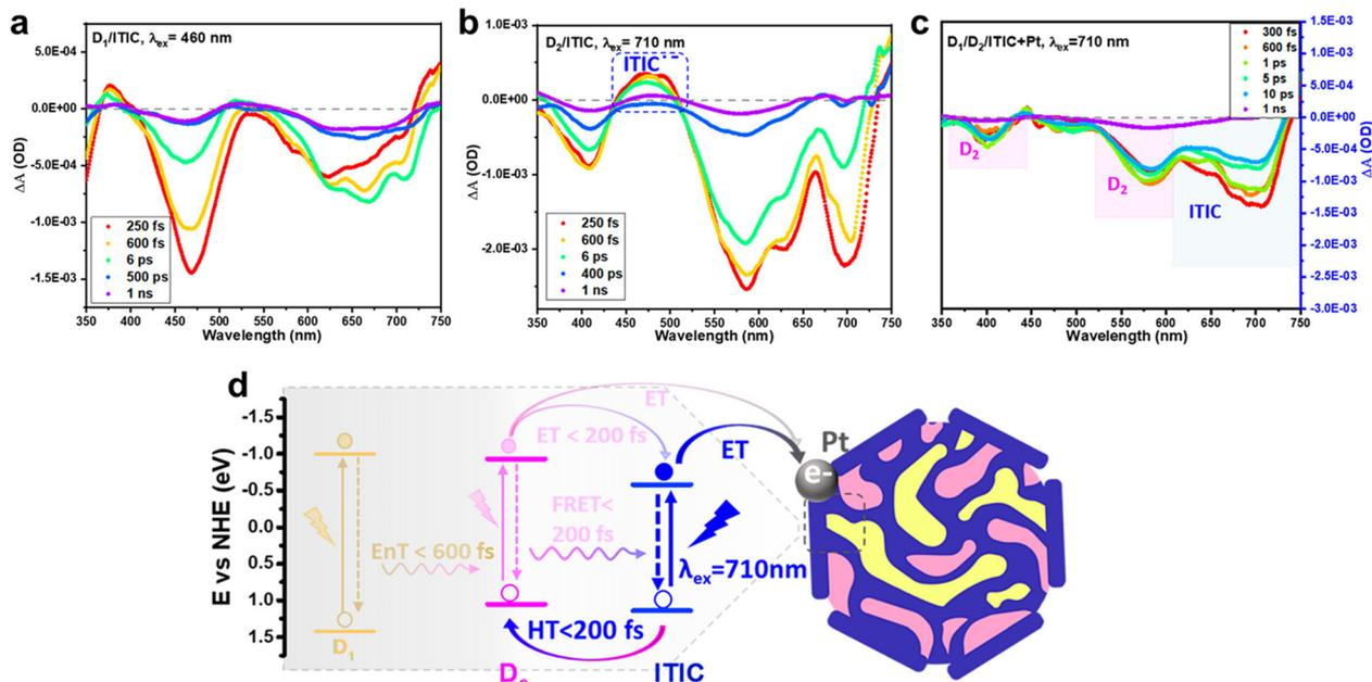
Fig. 11 Transient absorption spectra of the (a) D<sub>1</sub>/ITIC, (b) D<sub>2</sub>/ITIC, and (c) ternary D<sub>1</sub>/D<sub>2</sub>/ITIC nanoparticles without with Pt cocatalyst, at an excitation wavelength of 710 nm with fluence of 80 μW. (d) Schematic of the charge carrier pathways in the photocatalytic process involving ternary nanoparticles. Reproduced with permission.<sup>115</sup> Copyright 2021, ACS publication.
