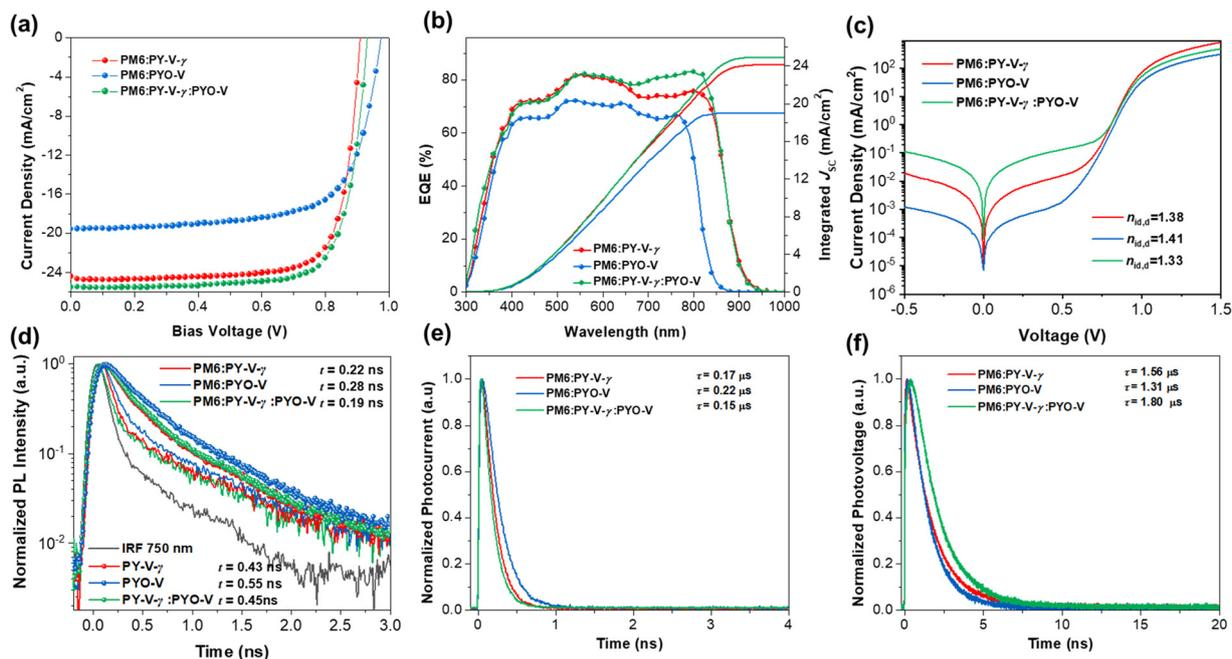
Fig. 2 (a)  $J$ - $V$  characteristics and (b) external quantum efficiency (EQE) spectra and (c) dark  $J$ - $V$  curves of the three types of all-PSCs. (d) TR-PL decay curves of the PY-V- $\gamma$ , PYO-V, and PY-V- $\gamma$ :PYO-V neat films and the PM6:PY-V- $\gamma$ , PM6:PYO-V and PY-V- $\gamma$ :PYO-V blend films. The pump and probe wavelengths are 750 nm. (e) TPC and (f) TPV spectra of the four all-polymer devices.
