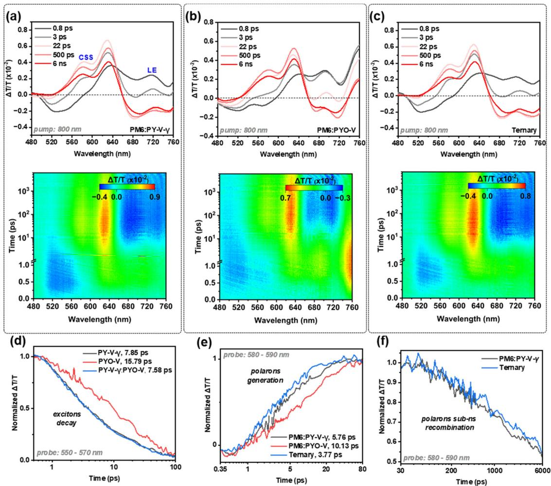
Fig. 4 (a)–(c) Spectral line cuts and pseudo-2D maps of transient absorption for acceptor and donor–acceptor blend thin films at a constant excitation fluence of  $2 \mu\text{J cm}^{-2}$  with an 800 nm pump wavelength. The corresponding kinetics are also plotted for (d) singlet exciton photo-induced absorption decay, (e) polaron photobleach generation, and (f) polaron recombination at a sub-ns regime.
