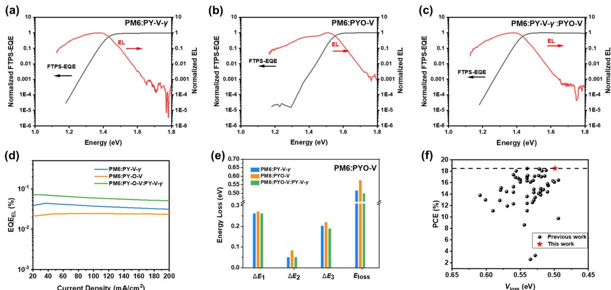
Fig. 5 (a)–(c) Semilogarithmic plots of normalized EL, measured EQE, and EQE calculated using FTPS (EQE-FTPS) as a function of energy for devices. (d) EQE<sub>EL</sub> spectra. (e) Detailed  $E_{\text{loss}}$  of devices. (f) All polymer  $V_{\text{loss}}$  vs. PCE.
