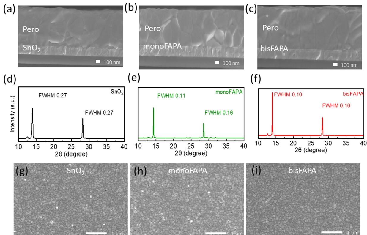
Fig. 3 (a)–(c) Cross-sectional SEM of perovskite on  $\text{SnO}_2$ , monoFAPA and bisFAPA modified  $\text{SnO}_2$  interfaces. (d)–(f) the XRD pattern of perovskite on bare  $\text{SnO}_2$  and two FAPA modified interfaces. (g)–(i) Top-view of perovskite on different interfaces after 3000 bending circles.
