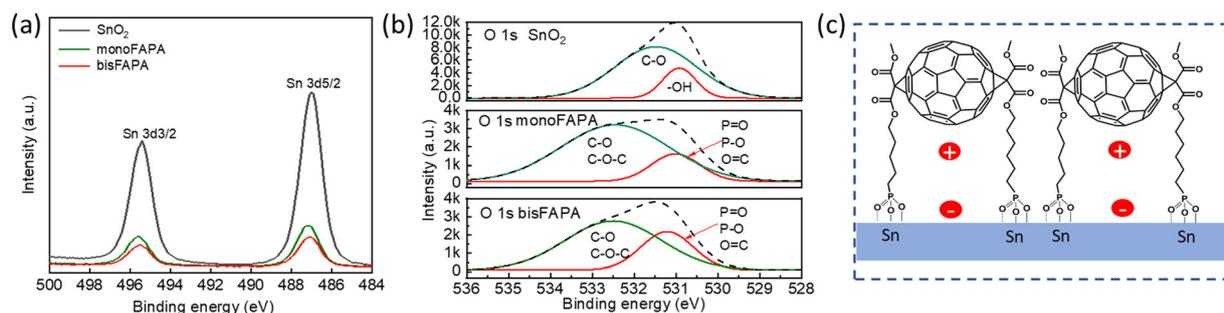
Fig. 4 (a) XPS spectra of Sn 3d. (b) O 1s XPS on thin films of  $\text{SnO}_2$ ,  $\text{SnO}_2$  modified with monoFAPA and bisFAPA, respectively. The dashed lines represent the raw data, while the solid lines represent the peak signal that has been fitted. The C–O peak on  $\text{SnO}_2$  surface likely stems from the ligands contained in the  $\text{SnO}_2$  nanoparticle ink. (c) Schematic illustration of bisFAPA bonding to the  $\text{SnO}_2$  surface.
