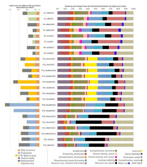
Fig. 7 Single scored weighted average cradle-to-grave LCA results for the bulk carrier (25 000 – 49 999) for the 24 technological pathways assessed. In the left side the results are separated into life cycle phases: well-to-tank (WTT), tank-to-wake (TTW), production of powertrain components, replacement of power train components, ship structure showing the contribution of each phase to the total score and right side shows the contribution of individual impact category
