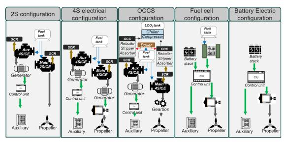
Fig. 3 Powertrain system configurations considered in the study from tank to wake
