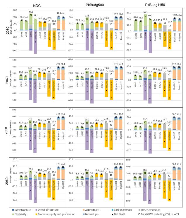
Fig. 12 Scenario analysis of GWP for production for different fuels. Negative emission for methanol and methane is due to the presence of carbon from biogenic origin or DAC in the fuel. The scenario is given for four decades from 2030 to 2060 during the period when the case study ship will be operating. (NH<sub>3</sub>-ammonia, LH<sub>2</sub>-liquid hydrogen, LMG-liquid methane, MeOH-methanol, ATR-auto thermal reforming, CC-carbon capture, and WTT-well to tank).
