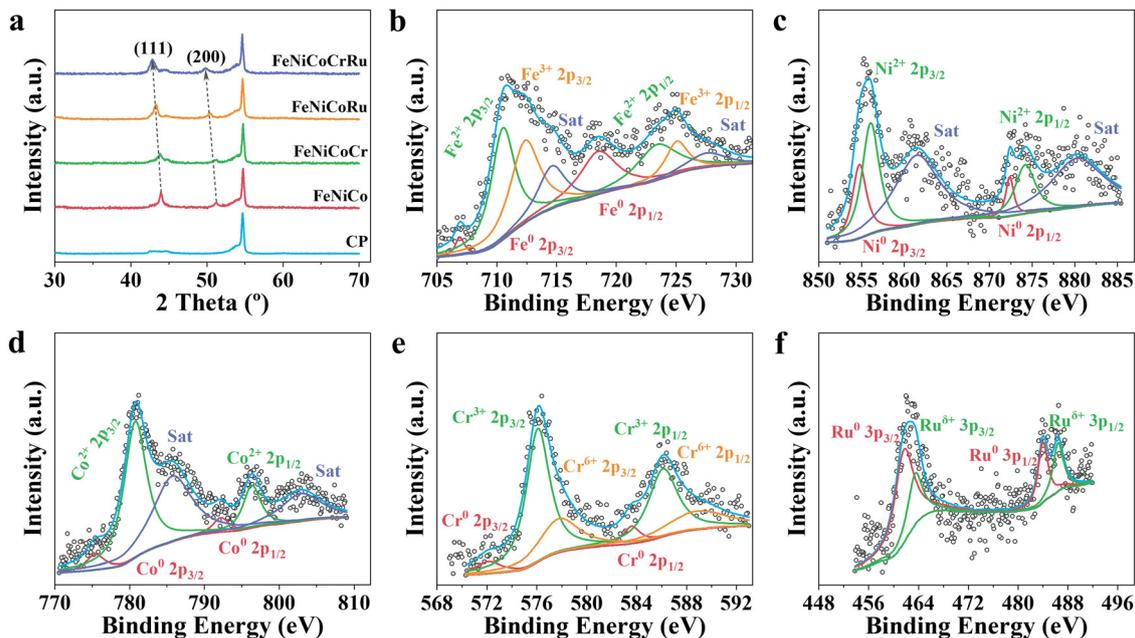
Fig. 2 (a) XRD spectra of FeNiCoCrRu, FeNiCoRu, FeNiCoCr, FeNiCo, and carbon paper (CP). High-resolution (b) Fe 2p, (c) Co 2p, (d) Ni 2p, (e) Cr 2p, and (f) Ru 3p spectra of FeNiCoCrRu HEA NPs.
