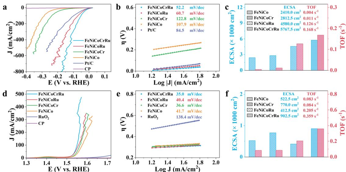
Fig. 3 Electrochemical water splitting performance of FeNiCoCrRu in 1 M KOH. LSV curves of (a) HER and (d) OER at a scan rate of 10 mV s<sup>-1</sup> with 95% *iR* compensation. Tafel slope plots of (b) HER and (e) OER. ECSA and TOF plots of (c) HER and (f) OER.
