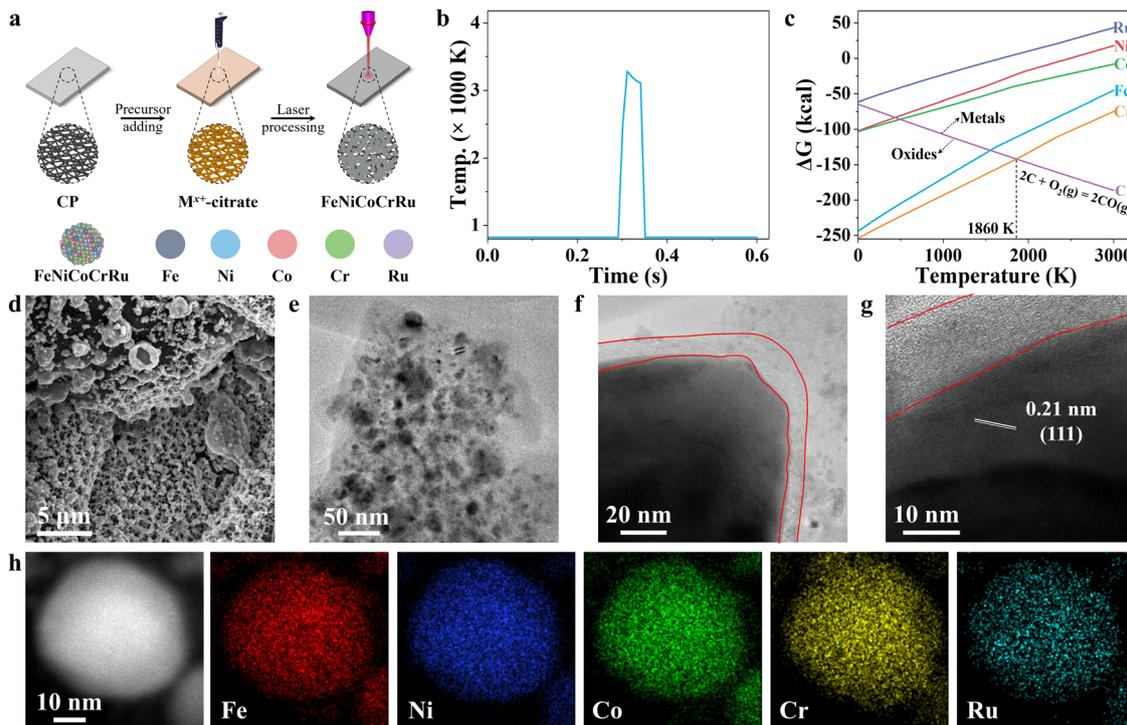
**Fig. 1** (a) Schematic showing the synthesis steps of FeNiCoCrRu HEA NPs using a CO<sub>2</sub> laser. (b) A temperature profile during CO<sub>2</sub> laser irradiation. (c) An Ellingham diagram showing the Gibbs free energies for the five metal elements as a function of temperature. (d) SEM, (e) TEM, (f)–(g) high-resolution TEM (HRTEM), (h) high-angle annular dark-field STEM (HAADF-STEM) and energy dispersive X-ray (STEM-EDX) elemental mapping images of HEA NPs.
