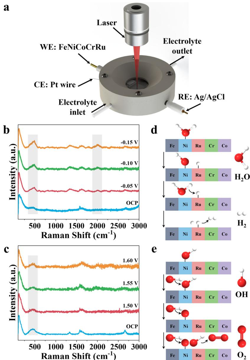
Fig. 5 (a) *In situ* Raman spectroscopy setup. *In situ* Raman spectra of the FeNiCoCrRu HEA at various potentials for (b) HER and (c) OER in 1 M KOH + 0.5 M NaCl electrolyte. Proposed catalytic mechanism of (d) HER and (e) OER in the alkaline seawater electrolyte.
