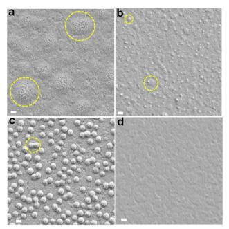
Fig. 2 SEM images ITO/bl-TiO<sub>2</sub> substrates after spin-coating DMF/DMSO dispersions (3.0 mg  $g^{-1}$ ) of (a) NG-60, (b) NG-100 and (c) NG-200 particles. An SEM of the bare ITO/bl-TiO2 substrate is shown in (d) for comparison. The yellow circles highlight coalesced nanogels. Scale bars: 200 nm.
