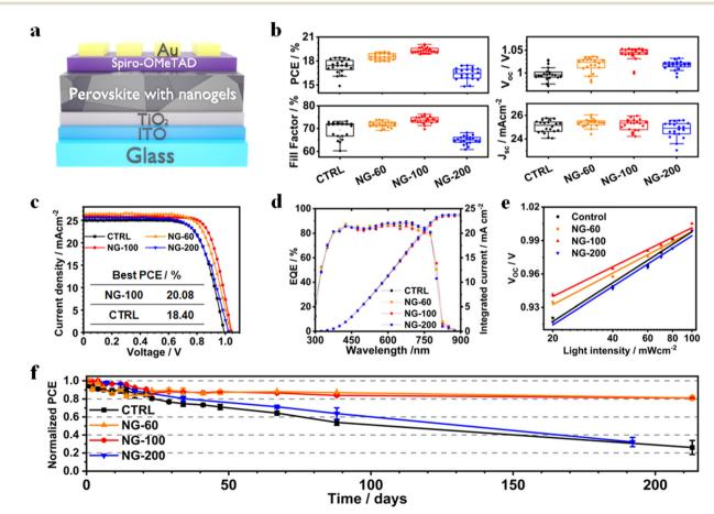
Fig. 4 (a) Device architecture used. (b) Measured PCEs, fill factors, open-circuit voltages and short-circuit current densities for the devices. (c) J-V curves for selected devices. (d) EQE data for the devices. (e) The variation of the open-circuit voltage with incident light intensity. (f) Normalized PCE shelf-life storage data for the PSCs. The unencapsulated devices were stored at room temperature in the dark under ambient conditions, RH = 35%.
