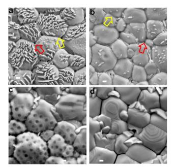
Fig. 3 Top view SEM images of the perovskite films prepared using (a) NG-60, (b) NG-100, (c) NG-200 and (d) the control without nanogels. The yellow arrows highlight nanofilm bridges between perovskite grains. The red arrows highlight small pinholes in the bridging nanofilms at the junction of three perovskite grains. Scale bars: 200 nm. See also Fig. S11 (ESI†).
