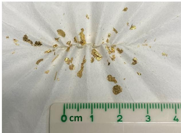
Fig. 6 Collected Au after filtration from filtrates.
