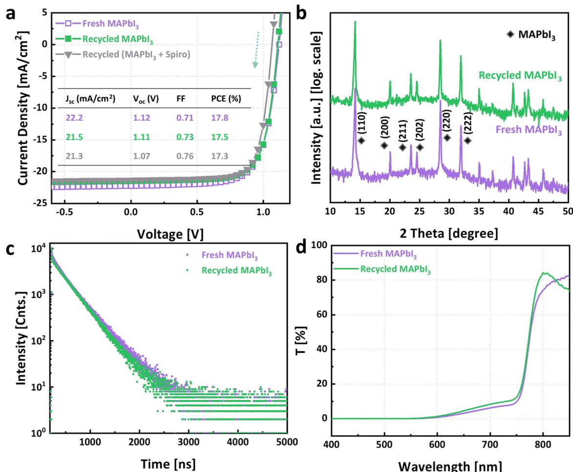
Fig. 4 Recycling of MAPbI<sub>3</sub>: (a) JV curves of perovskite solar cells using only fresh materials, recycled MAPbI<sub>3</sub>, and recycled MAPbI<sub>3</sub> and spiro-OMeTAD; (b) XRD patterns; (c) TR-PL spectra; (d) UV-Vis spectra of fresh and recycled MAPbI<sub>3</sub> films on common glasses.
