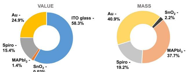
**Fig. 7** Value (left) and mass (right) composition of the investigated perovskite solar device. Note that the mass of the sample is dominated by that of the ITO glass, which per area weighs 1000 times more than all other materials combined.
