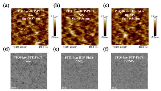
Fig. 6 AFM height images of without (a), CNPz (b), and DCNPz (c)-treated PTQ10:m-BTP-PhC6 blend films. TEM images of without (d), CNPz (e), and DCNPz (f)-processed PTQ10:m-BTP-PhC6 blend films.
