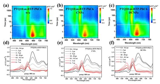
Fig. 5 fs-TAS measurement of PTQ10:m-BTP-PhC6 binary blends without/with different additives: (a)-(c) pseudo 2D color plots. (d)-(f) Spectral linecuts at the indicated pump-probe delay times. The samples were excited using an 800 nm fs-laser with 3 μJ cm<sup>-2</sup> fluence
