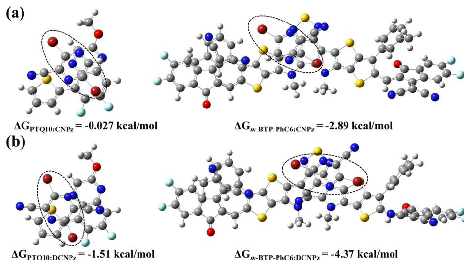
Fig. 3 The strongest conformations and calculated binding energies for the complexes of (a) PTQ10:CNPz, *m*-BTP-PhC6:CNPz and (b) PTQ10:DCNPz, *m*-BTP-PhC6:DCNPz.
