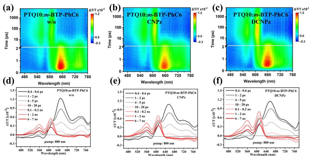
Fig. 5 fs-TAS measurement of PTQ10:*m*-BTP-PhC6 binary blends without/with different additives: (a)–(c) pseudo 2D color plots. (d)–(f) Spectral line-cuts at the indicated pump–probe delay times. The samples were excited using an 800 nm fs-laser with  $3 \mu\text{J cm}^{-2}$  fluence.
