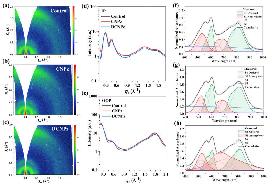
Fig. 7 2D GIWAXS patterns of PTQ10:*m*-BTP-PhC6 blend films: (a) control, (b) with CNPz additive and (c) with DCNPz additive. (d) and (e) The out-of-plane and in-plane line cut of the 2D GIWAXS data. Absorption profiles of PTQ10:*m*-BTP-PhC6 blend films without additive (f), with CNPz additive (g), and with DCNPz additive (h). White hollow point: experiment results; green shaded areas: ordered phase, red shaded areas: amorphous phase; dashed lines indicate vibronic sub-bands.
