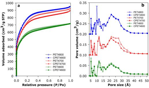
Fig. 3 Porosity of PET-derived activated carbon composites. (a) Nitrogen sorption isotherms and (b), pore size distribution (PSD) curves of PET-derived activated carbon composites before and after compaction at 370 MPa for 10 min. The PSD curves of PET4700 and CPET4700 are offset (y-axis) by 0.1, while those of PET4800 and CPET4800 are offset by 0.2.
