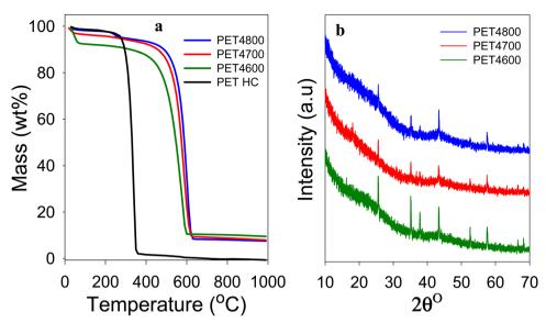
Fig. 1 Nature of PET-derived hydrochar and activated carbon composites. (a) TGA curves of PETHC hydrochar and PET4T activated carbon composites prepared at KOH/PETHC ratio of 4, and 600 –800 °C. (b) Powder XRD pattern of PET4T activated carbon composites prepared at KOH/PETHC ratio of 4, and 600-800 °C.
