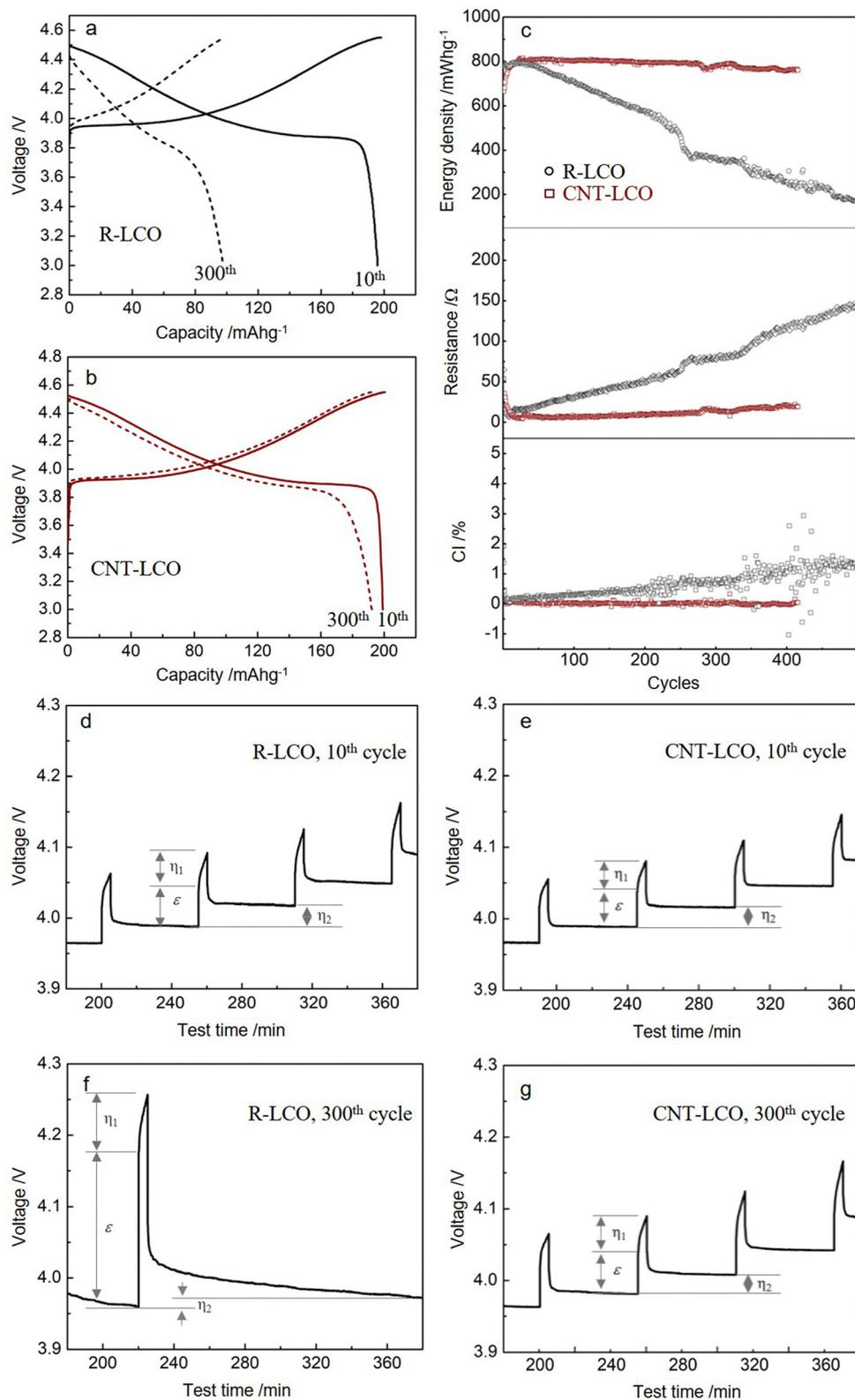
Fig. 2 Electrochemical performances of R-LCO and CNT-LCO. (a) and (b) Charge/discharge profiles of R-LCO and CNT-LCO at the 10<sup>th</sup> and 300<sup>th</sup> cycles between 3.0 and 4.55 V. (c) Cycling performances of the discharge energy density, Coulombic inefficiency, and interior resistance of R-LCO and CNT-LCO. (d)–(g) GITT profiles of R-LCO and CNT-LCO at the 10<sup>th</sup> and 300<sup>th</sup> cycles.
