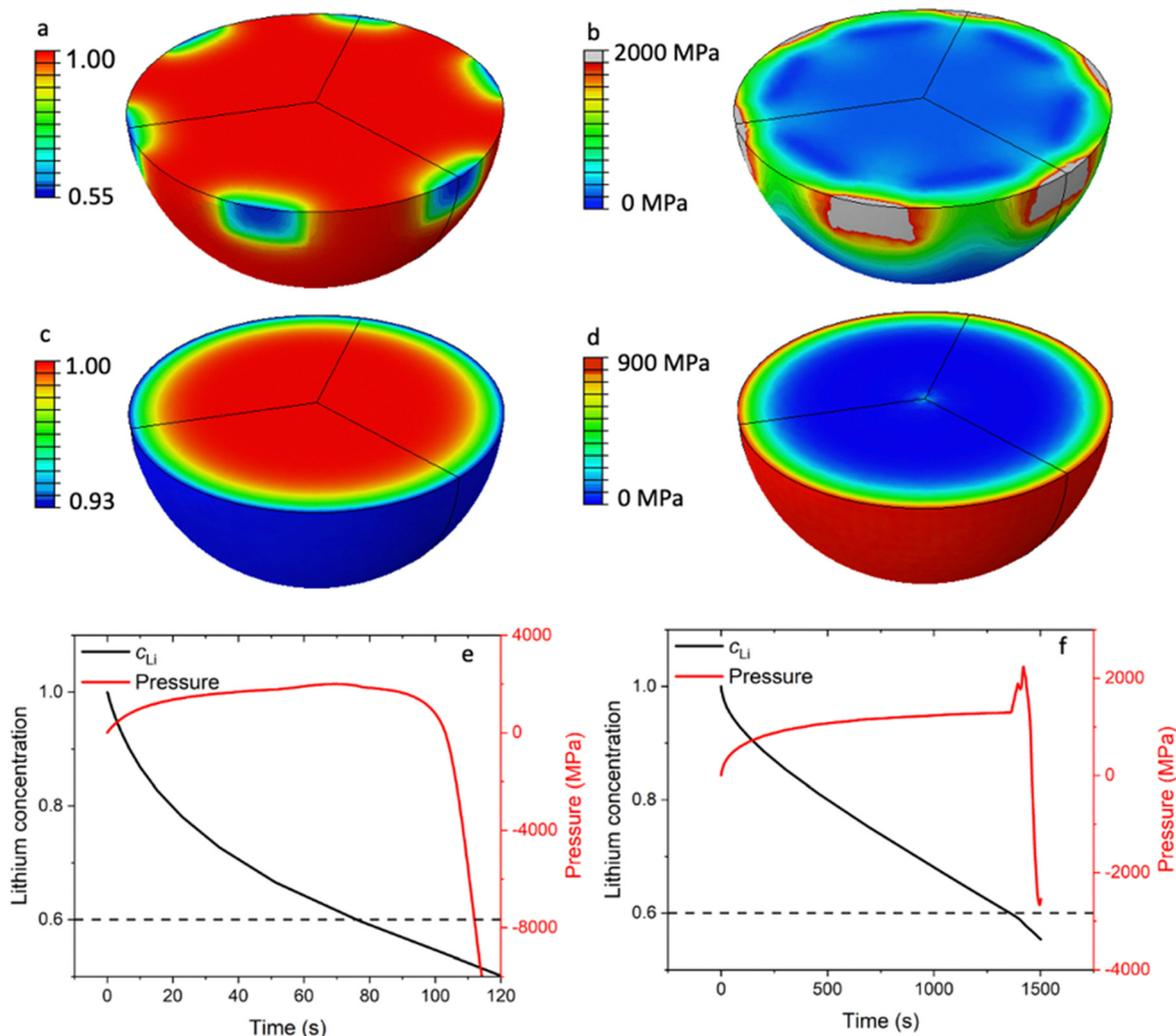
**Fig. 3** FEM simulations of the electrochemical indentation of R-LCO and CNT-LCO. (a) Li concentration in the LCO particle in R-LCO, (b) the von Mises stress field of LCO in R-LCO, (c) Li concentration in the LCO particle in CNT-LCO, (d) the von Mises stress field of LCO in CNT-LCO, (e) lithium concentration and pressure at a characteristic surface point in R-LCO and (f) the lithium concentration and pressure at a characteristic surface point in CNT-LCO.
