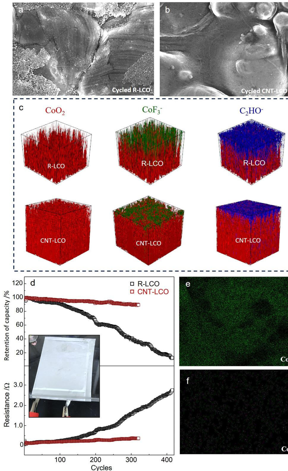
**Fig. 4** Particles after cycling and full-cell cycling performance. (a) and (b) SEM images of the LCO particles in R-LCO and CNT-LCO after high-voltage cycling. (c) TOF-SIMS analysis of the surface of the cycled R-LCO<sup>11</sup> and CNT-LCO electrodes. (d) Cycling performance of discharge energy retention and cell resistances of R-LCO and CNT-LCO full cells. (e) and (f) EDS mapping of Co on the graphite anode from the cycled R-LCO (e) and CNT-LCO (f) full cells.
