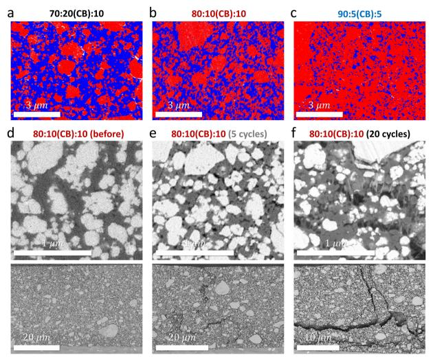
Fig. 3 The microstructure of the LMOF/CB/PVDF electrode before and after cycling. (a) -(c) The SEM-EDS maps of LMOF (red), CB/PVDF (blue), and pore (white) in the (a) 70:20:10, (b) 80:10:10, and (c) 90:5:5 electrodes before cycling. The cross-sectional samples were prepared with Argon ion milling. (d)-(f) The SEM images of the LMOF 80:10:10 electrode (d) before cycle, (e) after 5 cycles, and (f) after 20 cycles [1.5-4.8 V, 25 mA g-AM-1]: LMOF (white), CB/PVDF (gray), and pores (black).
