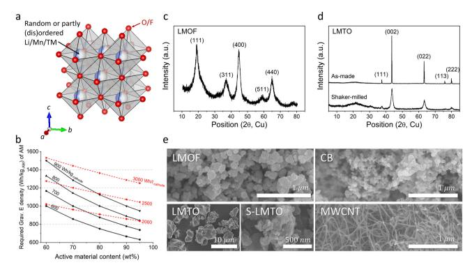
Fig. 1 Structure of components in Mn-DRX cathodes. (a) Schematic of the crystal structure of Mn-DRX. (b) The required gravimetric energy density (W h kg\_ahm\_1) in Mn-DRX to achieve various target cathode energy densities (W h kg\_cathode\_1, W h l\_cathode\_1) as a function of the AM content. The XRD patterns of (c) LMOF and (d) LMTO (before and after shaker-milling). (e) SEM images of LMOF, LMTO, shaker-milled LMTO (S-LMTO), carbon black (CB), and multiwalled carbon nanotube (MWCNT)
