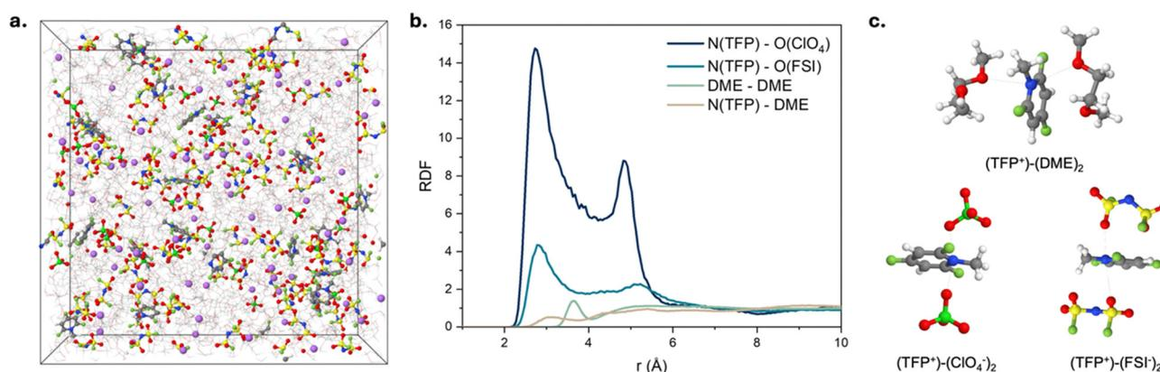
Fig. 4 (a) A snapshot of the MD simulation cell for 0.91 M LiFSI and 0.27 M [TFP]<sup>+</sup>[ClO<sub>4</sub><sup>-</sup>] in DME. (b) Radial distribution functions for 0.91 M LiFSI and 0.27 M [TFP]<sup>+</sup>[ClO<sub>4</sub><sup>-</sup>] in DME at 298 K and (c) representative cation solvates for 0.91 M LiFSI and 0.27 M [TFP]<sup>+</sup>[ClO<sub>4</sub><sup>-</sup>] in DME at 298 K.
