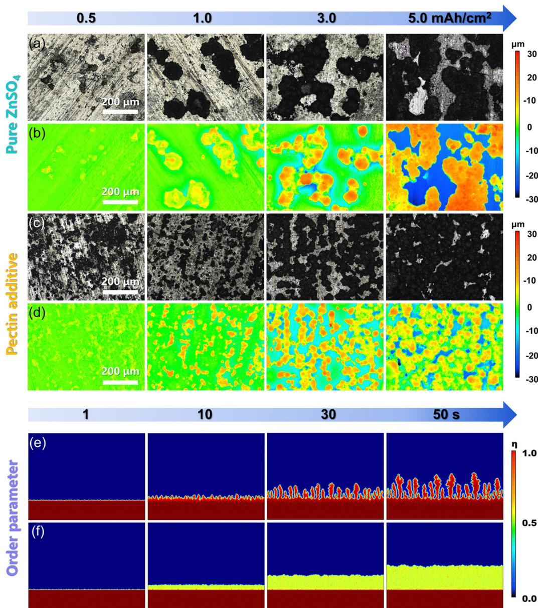
Fig. 2 Zn nucleation and deposition process. (a) and (c) CLSM optical images and (b) and (d) corresponding height images of Zn deposition with different capacities from 0.5 to  $5.0 \text{ mA h cm}^{-2}$  in the pure  $\text{ZnSO}_4$  and the electrolyte with pectin additive. COMSOL simulation of the morphology evolution on Zn anode using (e) pure  $\text{ZnSO}_4$  and (f)  $\text{ZnSO}_4$ -pectin after Zn electrodeposition for 1, 10, 30 and 50 s, respectively.
