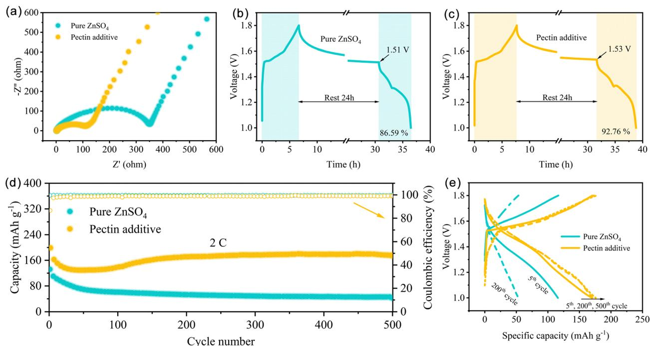
Fig. 6 The electrochemical performance of Zn||MnO<sub>2</sub> full cells. (a) Nyquist plots. (b) and (c) Self-discharge tests after a rest of 24 h. (d) Long-term cycling performance at 2C and (e) the corresponding charge–discharge curves.
