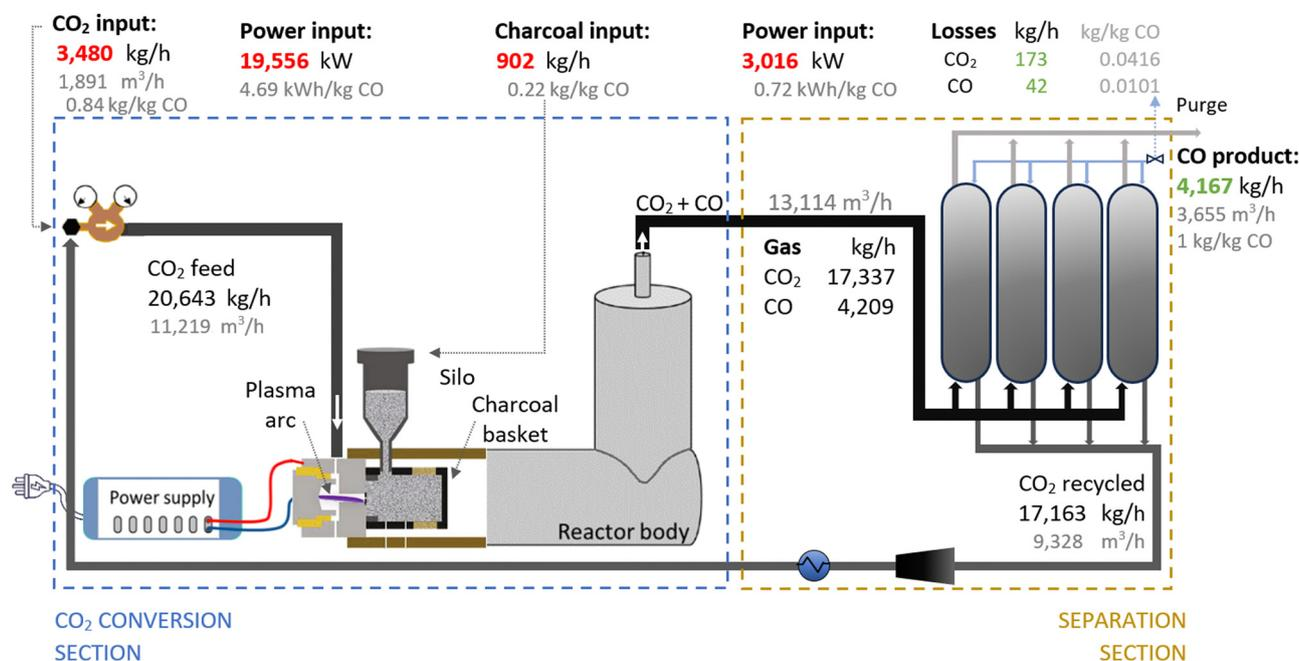
**Fig. 2** Schematic flowchart for the plasma-based plant, producing 100 tonnes CO per day. Carbon bed design based on Girard-Sahun *et al.* (2022).
