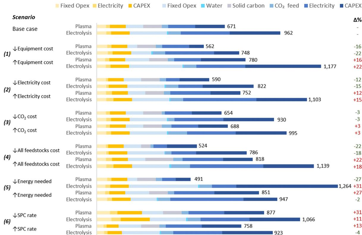
Fig. 5 Scenarios for sensitivity analysis of CO production costs. Values on the right of the bars represent the UCOP [\$ per tonne CO], and numbers in green and red in the right represent the percentage variation of the UCOP with respect to the base cases. Legends' colours are the same as those in Fig. 4. The underlying data for this chart is detailed in Table S5 of the ESI.†
