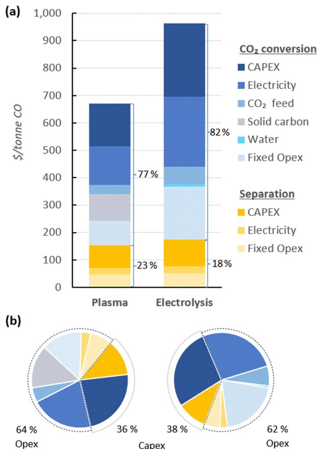
Fig. 4 Production costs of CO via plasma- and electrolysis-based plants. Chart (a) represents the costs aggregated by CO<sub>2</sub> conversion and separation sections (blue and yellow, respectively), and (b) represents the same contributions, with distinction between Capex and Opex (solid and dashed circle lines, respectively) to the total production cost. The underlying data for these charts is detailed in Table S5 of the ESI.†
