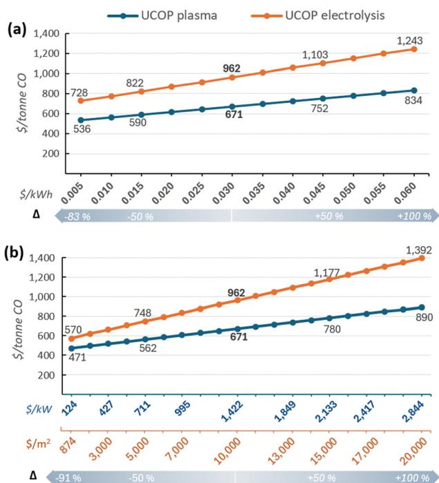
Fig. 6 Sensitivity analysis: (a) Electricity cost vs. UCOP of CO; (b) CO<sub>2</sub> conversion equipment cost vs. UCOP of CO. Values on the X-axis in blue represent the cost of the plasma system (\$ per kW), while values in orange represent the cost of the electrolyser (\$ per m<sup>2</sup>). The underlying data for these charts are detailed in Tables S6 and S7 of the ESI.†
