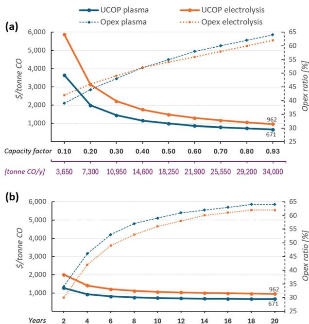
Fig. 7 Sensitivity analysis: (a) Capacity factors vs. UCOP of CO; (b) CO<sub>2</sub> conversion equipment lifespan vs. UCOP of CO. Solid lines represent UCOP of CO (left Y-axis), while dashed lines represent the ratio of Opex to UCOP of CO (right Y-axis). The underlying data for these charts are detailed in Tables S8 and S9 of the ESI.†
