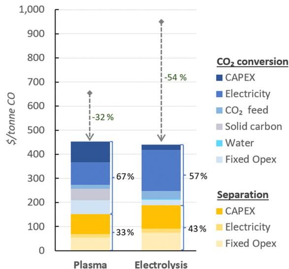
Fig. 8 Optimal scenario for alternative CO production plants. The values next to the bars indicate the contribution of CO<sub>2</sub> conversion and separation sections to the UCOP, while the values on top of the bars represent the percentage variation relative to the UCOP of the base cases.
