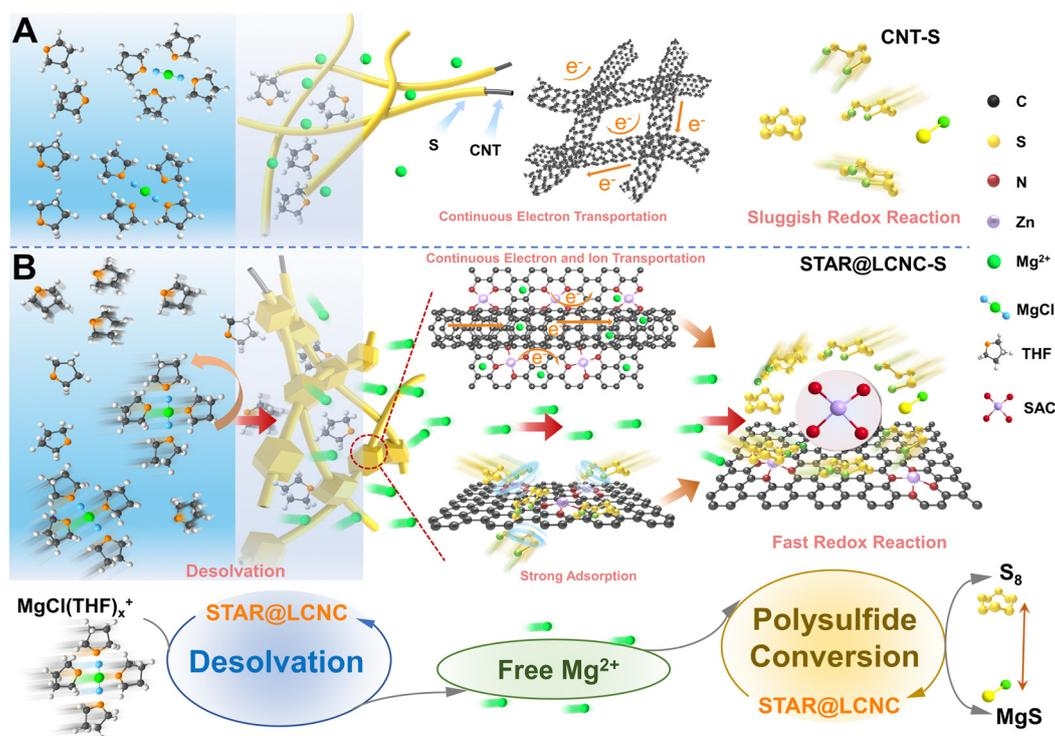
**Fig. 1** Schematic illustrations of atomic reactors in triphasic interfaces. The schematic illustrations of (A) electronic transport along the cross-linked CNT and (B) fast electronic transport, strong chemisorption, and rapid conversion kinetics of magnesium polysulfides at the solid–liquid–solid ternary interfaces with the catalysis of atomic reactors.
