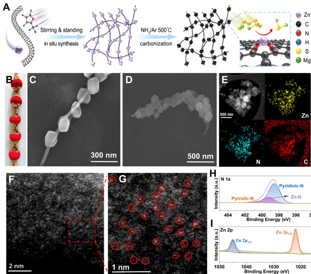
**Fig. 3** Synthesis and characterizations of the STAR@LCNC catalyst. (A) A schematic synthesis illustration of the STAR@LCNC. (B) An optical image of a Chinese lantern. SEM images of (C) ZIF-8/CNT and (D) STAR@LCNC samples. (E) The energy dispersed X-ray elemental mappings of C, Zn and N in STAR@LCNC. (F) and (G) HAADF-STEM images of the single zinc atoms in the STAR@LCNC composite (highlighted by circles in (G)). High-resolution XPS spectra of (H) N 1s and (I) Zn 2p of STAR@LCNC.
