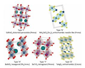
Fig. 2 Perovskite structure of the chalcogenide ABX<sub>3</sub>. The cell diagram of the crystal structure of chalcogenide perovskites, as well as their geometric shape, space group, and prototype composition. <sup>82</sup> Copyright 2021 Devendra Tiwari *et al.* J. Phys. Energy.
