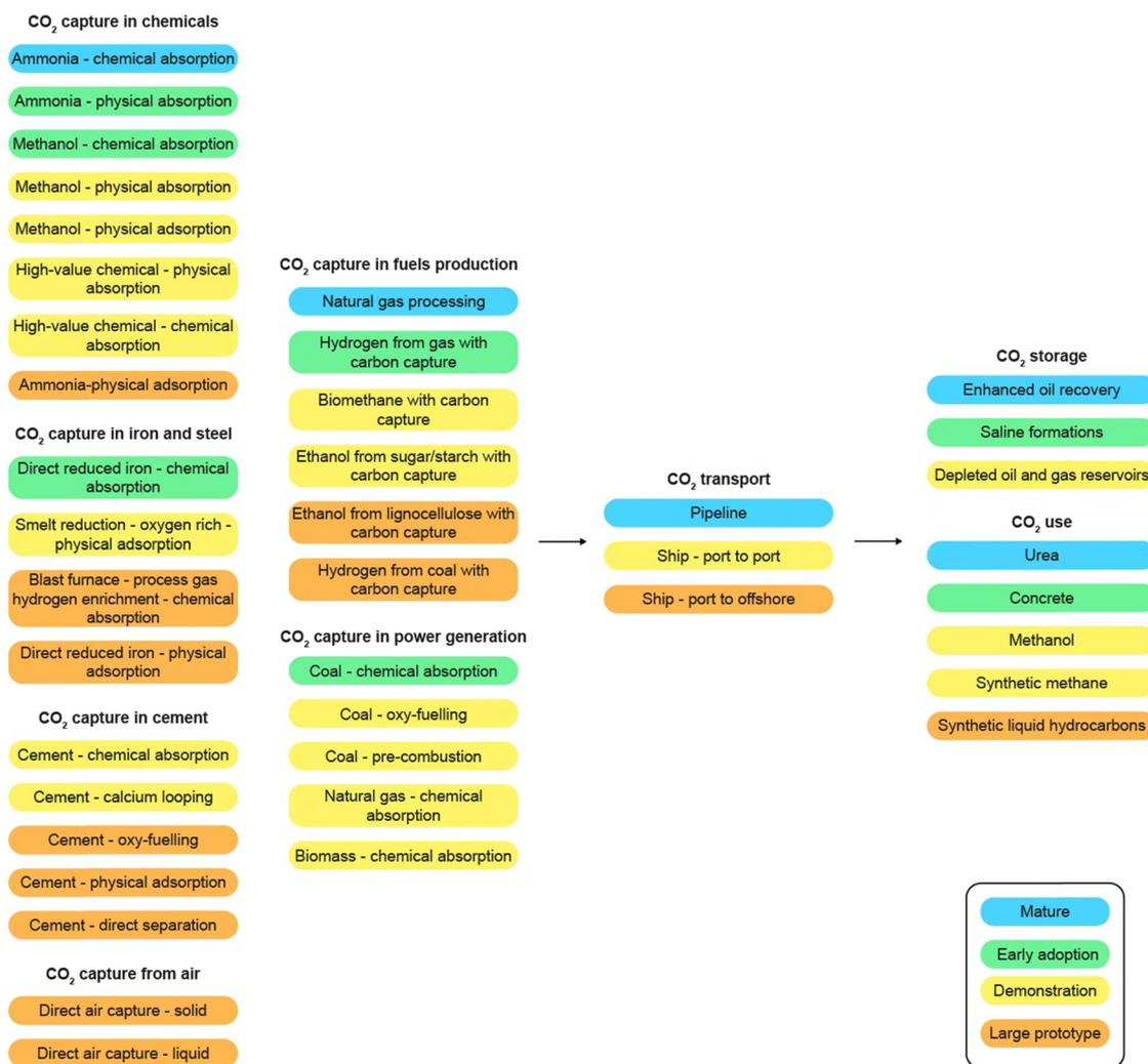
Fig. 4 The technology readiness level (TRL) of multiple technologies along the CCUS value chain. Source, retrieved from ref. 244.
