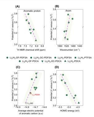
Fig. 4 Correlation between the chemical shift of the aromatic proton (A), and the shift of the aromatic band in the FTIR spectra (B) with the delithiation potential of the studied chemistries. Correlation between the average electric potential of aromatic carbon (C; Li<sub>2</sub>-BQ<sup>16</sup> and Li<sub>2</sub>-PDSA<sup>17</sup> were used as benchmark systems), and the HOMO (D) with the delithiation potential of the studied materials
