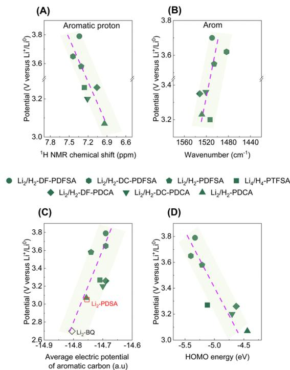
**Fig. 4** Correlation between the chemical shift of the aromatic proton (A), and the shift of the aromatic band in the FTIR spectra (B) with the delithiation potential of the studied chemistries. Correlation between the average electric potential of aromatic carbon (C;  $\text{Li}_2$ -BQ<sup>16</sup> and  $\text{Li}_2$ -PDSA<sup>17</sup> were used as benchmark systems), and the HOMO (D) with the delithiation potential of the studied materials.
