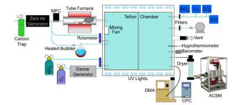
Fig. 1 Experimental laboratory schematic adopted from Pokhrel et al.  $^{60}$  Particle aging was studied in a 9.0 m $^3$  smog chamber at the North Carolina Agricultural and Technical State University (NC A&T University). The setup features a tube furnace that allows temperature control, where  $\sim 0.050-0.50$  gram fuel samples were combusted at 450 °C. The chamber has been fully characterized in a prior study. $^{66}$
