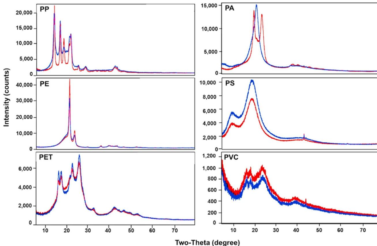
Fig. 11 XRD pattern of PP, PE, PET, PA, PS, and PVC; red refers to small particles and blue refers to large particles (License: Under Creative Commons CC-BY).<sup>51</sup>
