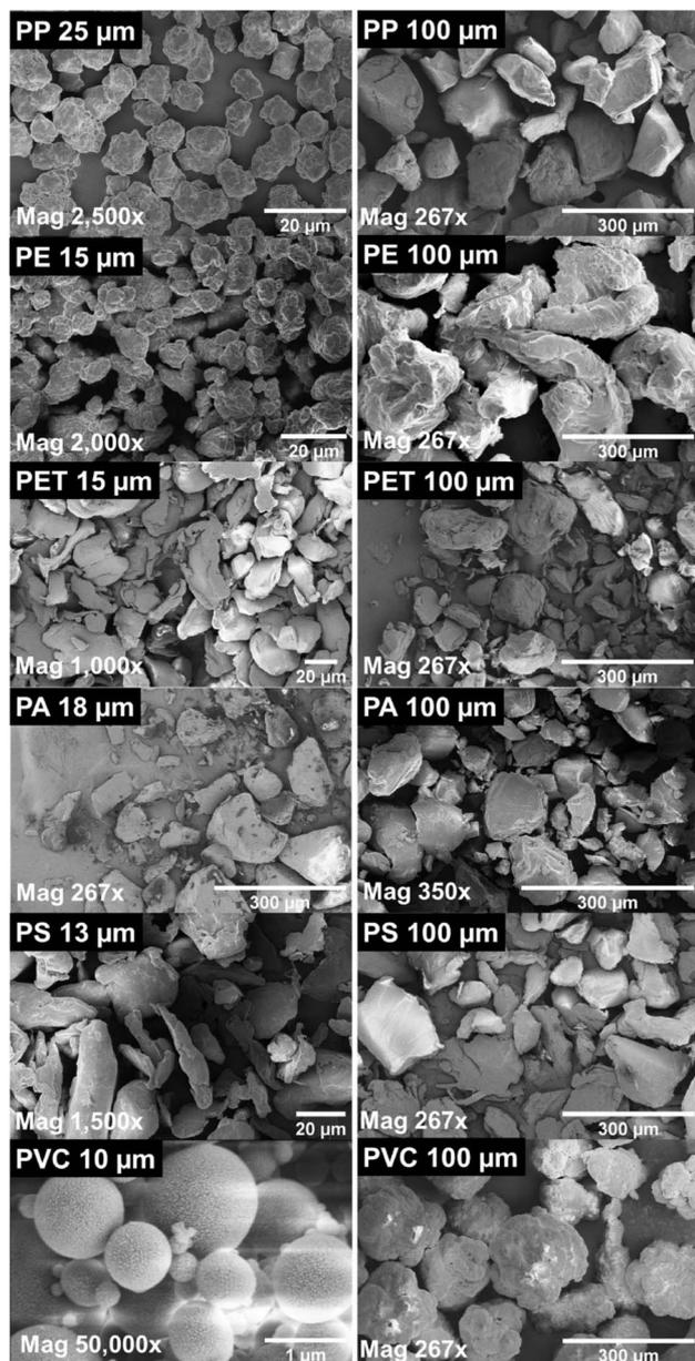
Fig. 12 SEM images of PP, PE, PET, PA, PS, and PVC with the magnification of the images ranging from 297 $\times$  to 50 000 $\times$  (License: Under Creative Commons CC-BY).<sup>51</sup>
