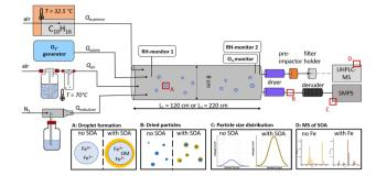
Fig. 1 Summary of experimental set-up and schematic representation of observations
