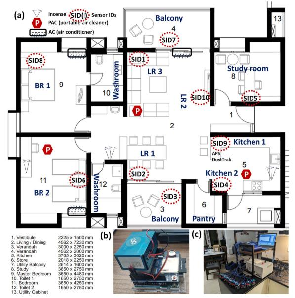
Fig. 1 (a) Layout of the apartment showing the locations of ten low-cost air quality monitors (LCAQMs), air conditioners (ACs), portable air purifier (PAC), and emission sources, (b) Plantower PMS5003-based LCAQMs; and (c) the collocation of all the LCAQMs along with the APS and DustTrak. Floor plan layout adapted from the campus plan document (https://campus.iitqn.ac.in/pdf/Design-of-Housing.pdf).
