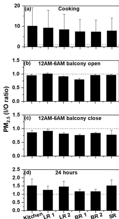
Fig. 6  $PM_{2.5}$  indoor to outdoor ( $I/O$ ) ratio calculated for different zones of the apartment during (a) cooking, (b) 12 AM–6 AM with open balconies, (c) 12 AM–6 AM with closed balconies, and (d) over entire 24 hours (midnight–midnight).
