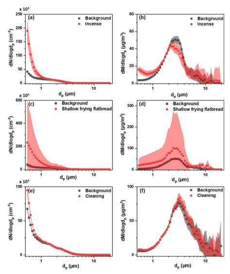
Fig. 2 The left panel shows the particle number size distribution (PNSD), and the right panel shows the particle mass size distribution (PMSD) corresponding to three sources: (a and b) incense, (c and d) cooking, and (e and f) cleaning.
