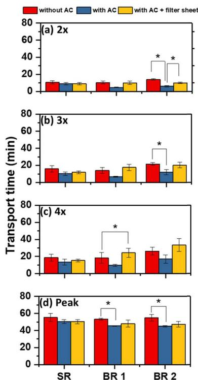
Fig. 3 Time for the concentrations in the study room (SR), bedroom 1 (BR 1), and bedroom 2 (BR 2) to reach (a) 2 $\times$ , (b) 3 $\times$ , (c) 4 $\times$ , and (d) peak relative to the background concentration under three scenarios: without AC, with AC on, and with AC on + filter sheet, \* with bracket shows the compared categories and presence of significance difference.
