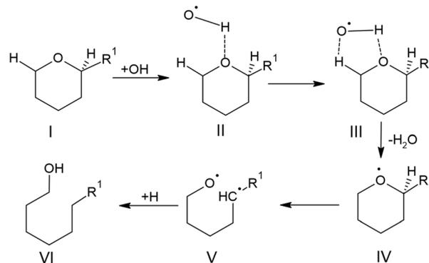
**Scheme 4** Possible mechanism for the ring opening of a substituted tetrahydropyran (oxane) structure. A plausible ring opening of similar structures in HAB toxins such as those in ciguatoxins, brevetoxins, palytoxins, and okadaic acids. Larger rings are more likely to open because of less steric hindrance for  $\cdot\text{OH}$  attack.
