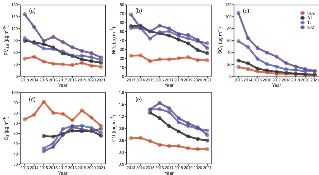
Fig. 4 Annual averages of PM<sub>2.5</sub> (a), NO<sub>2</sub> (b), SO<sub>2</sub> (c), O<sub>3</sub> (d), and CO (e) at SDZ, BJ, TJ and SJZ during 2013–2021, respectively.
