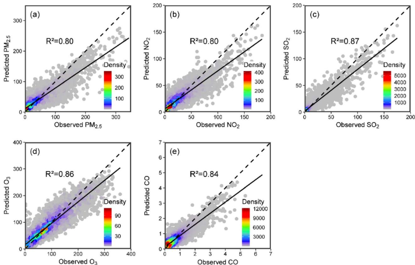
Fig. 2 Correlations between the hourly observed and predicted data on the testing datasets of  $\text{PM}_{2.5}$  (a),  $\text{NO}_2$  (b),  $\text{SO}_2$  (c),  $\text{O}_3$  (d), and CO (e). The units of  $\text{PM}_{2.5}$ ,  $\text{NO}_2$ ,  $\text{SO}_2$ , and  $\text{O}_3$  are  $\mu\text{g m}^{-3}$ , while that of CO is  $\text{mg m}^{-3}$ .
