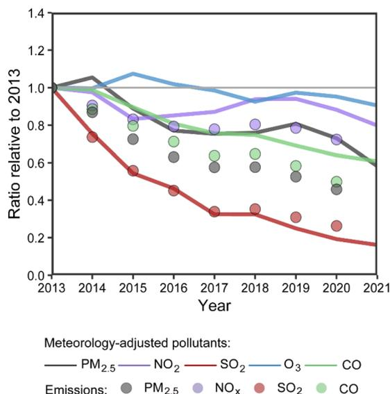
Fig. 6 Normalized trend of the meteorology-adjusted air pollutant concentrations at SDZ and emissions of PM<sub>2.5</sub>, NO<sub>2</sub>, SO<sub>2</sub> and CO. The emission data during 2013–2021 were obtained from <https://meicmodel.org/>.
