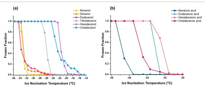
Fig. 4 The frozen fraction of (a) fatty alcohols and (b) fatty acids relative to the temperature at which the individual droplets underwent freezing.
