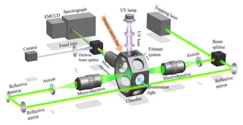
Fig. 1 Schematic of the experimental setup of the OT-RS system.
