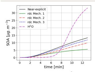
Fig. 1 Toluene SOA concentrations (in  $\mu g\ m^{-3}$ ) simulated with different toluene SOA mechanisms (the near-explicit mechanism Mech. 2, the reduced mechanisms rdc. Mech. 1, rdc. Mech. 3 and H<sup>2</sup>O) for the flow tube experiment of Lannuque et al.39
