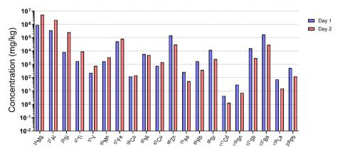
Fig. 7 ICP-MS results for two separate days, denoted with blue and red, including only submicron TRWPs.
