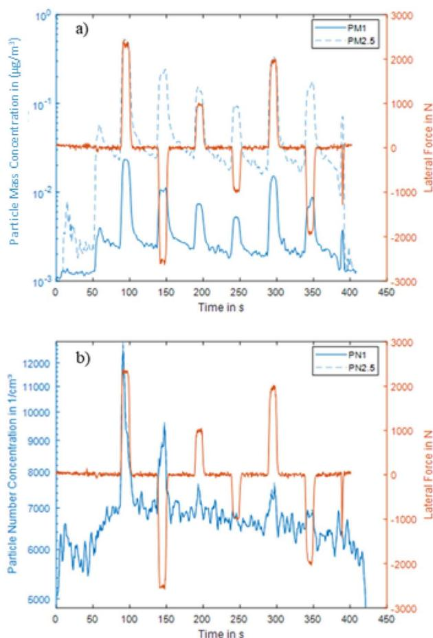
Fig. 5 The steady-state force (right axis, orange) is shown with particle concentration (left, blue) for (a) PM and (b) PN measurements for submicron particles ( $PN_1$  solid line) and up to 2.5 microns ( $PM_{2.5}$  dotted line). The  $PN_{2.5}$  and  $PN_1$  lines are indistinguishable as they overlap.
