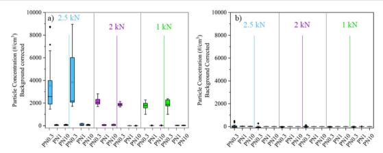
Fig. 6 Box and whisker plot for steady-state cycle data shown for repeat cycles for PN (a) without the CS (representative of all particles) and (b) with the CS (only the solid, non-evaporative particles). The data are grouped for particle sizes  $0.006-0.26 \,\mu m$  (PN<sub>0.3</sub>),  $0.26-1 \,\mu m$  (PN<sub>0.3-1</sub>), and  $1-10 \,\mu m$  (PN<sub>1-10</sub>). The analysis is shown for 2.5 kN (blue), 2 kN (purple), and 1 kN (green) forces.
