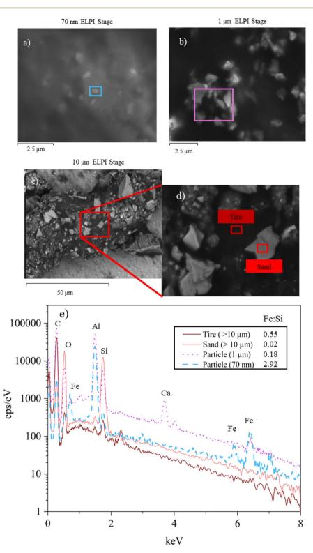
Fig. 8 SEM images for the chemical composition of (a) a 70 nm stage particle (blue) and background (grey), (b) a 1  $\mu$ m stage particle (purple) and (c) a >10  $\mu$ m stage particle highlighting the (d) tire (maroon) and sand (red) components. The EDX spectrum is shown (e) with present elements noted.
