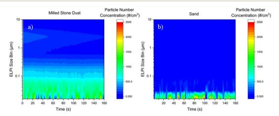
Fig. 2 Particle size distribution by concentration (colour bar) shown for (a) milled stone dust and (b) sand at a constant tire speed of 50 kilometres per hour.
