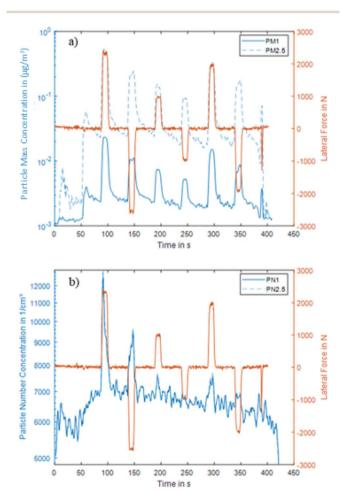
Fig. 5 The steady-state force (right axis, orange) is shown with particle concentration (left, blue) for (a) PM and (b) PN measurements for submicron particles (PN $_1$  solid line) and up to 2.5 microns (PM $_{2.5}$  dotted line). The PN $_{2.5}$  and PN $_1$  lines are indistinguishable as they overlap.
