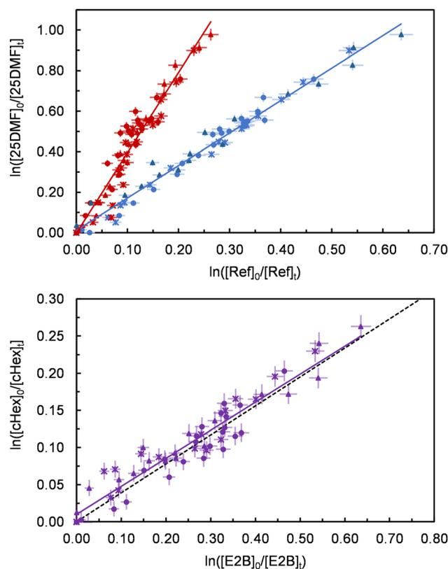
Fig. 1 Relative-rate plots of the 2,5-dimethylfuran + O<sub>3</sub> system using cyclohexene (red) and E2-butene (blue) as references (upper panel) and the crosscheck of both references (lower panel) using the PTR-MS data. The dotted line represents the theoretically expected rate coefficient ratio. Different experimental runs are denoted with different symbols. Error bars represent the  $2\sigma$  statistical uncertainty.
