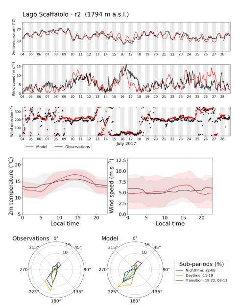
Fig. 4 Modeled (red lines) and observational (black lines) data for the station of Lago Scaffaiolo (r2). Top panels report the timeseries of air temperature ( $^{\circ}$ C), wind speed (ms $^{-1}$ ) and direction ( $^{\circ}$ ). Bottom panels report the corresponding average diurnal cycle and wind direction frequencies for the same period, as in Fig. 2.
