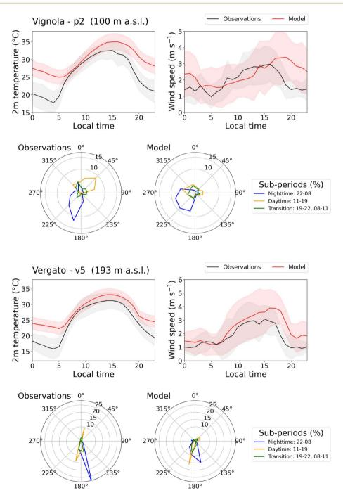
Fig. 3 Modeled (red lines) and observational (black lines) data as in Fig. 2 but for the stations of Vignola (p2) and Vergato (v5).
