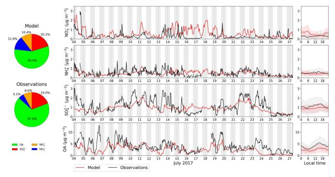
Fig. 6 Pie charts, (left), timeseries (centre) and diurnal cycles (right) of the observed (black) and modeled (red)  $PM_1$  chemical components ( $NO_3^-$ , NH<sub>4</sub><sup>+</sup>, SO<sub>4</sub><sup>2-</sup>, OA) during the investigated period (4th-27th July 2017). Centre and right panels share the y axis (different between inorganic and organic components). Shaded areas represent nights.
