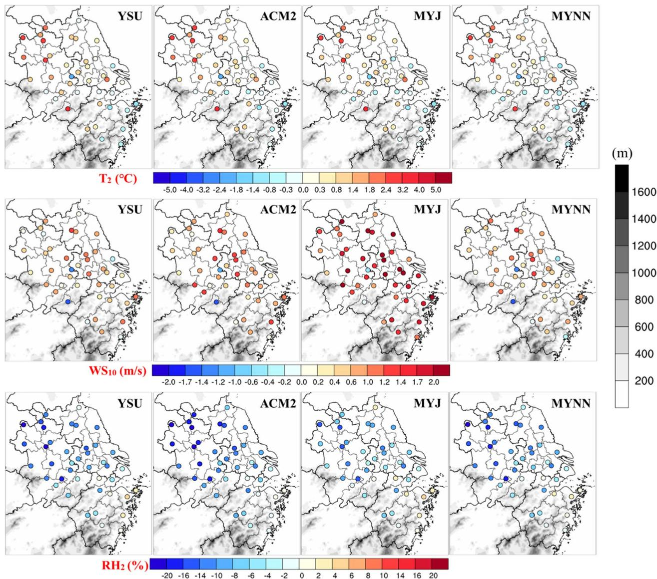
Fig. 6 Model bias (MB) of  $T_2$ ,  $WS_{10}$ , and  $RH_2$  in 41 cities of the YRD region in July 2018.
