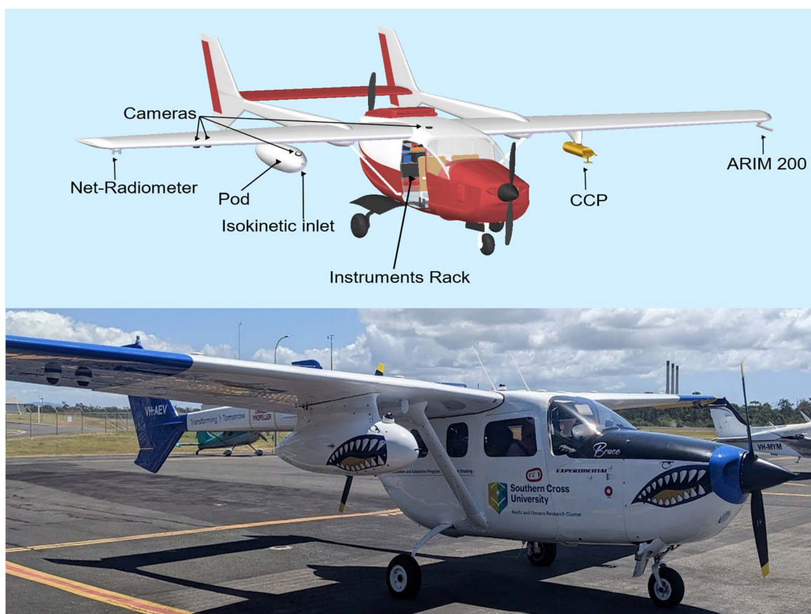
Fig. 1 Conceptual design of the aircraft sampling platform showing major external instrumentation and photo of the final configuration.
