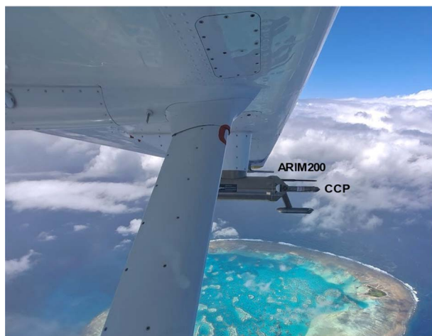
Fig. 3 Photo of left-hand underwing probes showing the mounting of the Cloud Combination Probe (CCP) from Droplet Measurement Technologies (DMT) and the ARIM200 Air Data Probe (ADP) from Aventech.
