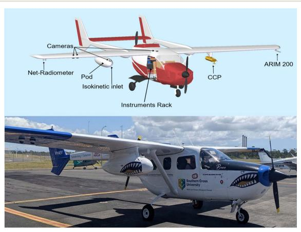
Fig. 1 Conceptual design of the aircraft sampling platform showing major external instrumentation and photo of the final configuration.
