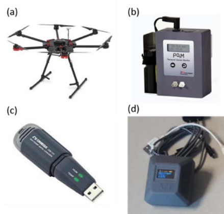
Fig. 2 The experimental system included the (a) DJI Matrice 600 Pro, (b) 2B Personal Ozone Monitor, (c) OM-141 temperature and humidity data logger, and (d) APT MINIMA particle sensor.
