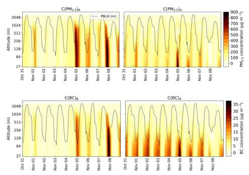
Fig. 9 Modelled vertical evolution of changes in total PM<sub>2.5</sub> (top) and BC (bottom) concentrations over Delhi due to the exclusion of anthropogenic and BB emissions as compared to the Base scenario during the study period. The dashed line in the top panels denotes the hourly variation of the modelled planetary boundary layer (PBL) height (identical in all sensitivity runs).
