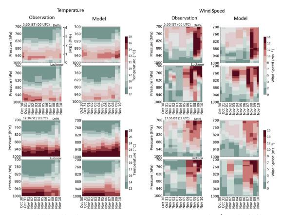
Fig. 8 Altitudinal variation (1000 to 700 hPa) of observed and simulated temperature and wind speed (m s<sup>-1</sup>) at 5:30 LT (IST) (top panel) and 17:30 LT (bottom panels) during the pollution episode. The observations are obtained from radiosonde profiles at Delhi and Lucknow, in the middle and lower IGP regions, respectively, as shown in Fig. 1.
