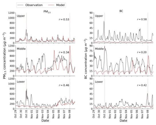
Fig. 2 Comparison of modelled (red) and observed (black) hourly mean concentrations of  $PM_{2.5}$  (left) and BC (right) averaged across the network of ground measurement sites (CPCB, IMD respectively) in the upper, middle and lower IGP regions. The vertical dashed lines in each panel delineate the pollution episode, and the r values are the Pearson's correlation coefficients.
