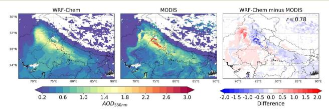
Fig. 3 Modelled and MODIS retrieved AOD $_{550nm}$  sampled at overpass times of 10.30 (Terra) and 13.30 (Aqua) and averaged over the pollution episode. The right panel shows the absolute differences between the model and satellite values (with a % difference plot shown in Fig. S6†), and r is the Pearson's correlation coefficient.
