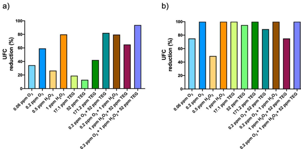
Fig. 4 Percentage of UFC reduction of airborne (a) bacteria and (b) fungi with triethylene glycol (TEG), ozone (O<sub>3</sub>) and hydrogen peroxide (H<sub>2</sub>O<sub>2</sub>) nebulized individually and combined. Plots represent percentage of reduction relative to the bacteria and fungi present before the nebulization of the compounds.
